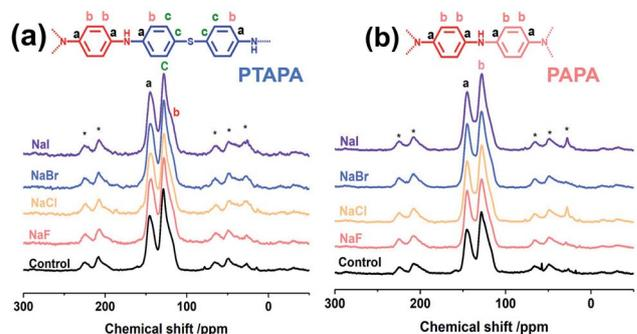
Fig. 2 SS <sup>13</sup>C NMR spectra of PTPA (a) and PAPA (b) before and after tuning by BXJ-salts.
