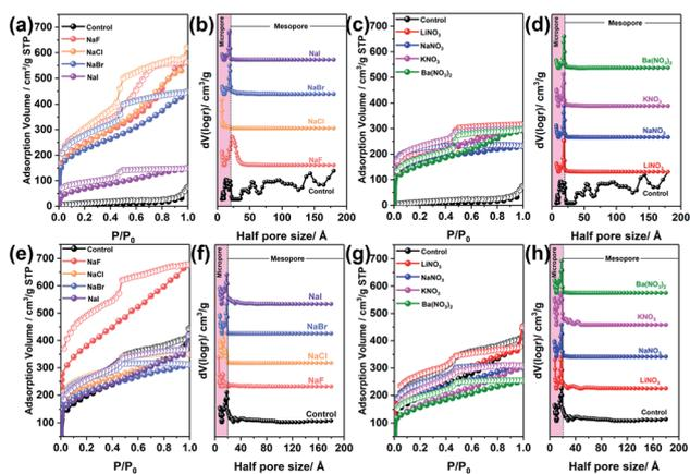
Fig. 3  $N_2$  adsorption and desorption isotherm and nonlocal density functional theory-pore size distribution of **PTAPA** ((a) and (b), tuned by BXJ sodium salts; (c) and (d), tuned by BXJ-nitrate salts) and **PAPA** ((e) and (f), tuned by BXJ sodium salts; (g) and (h), tuned by BXJ nitrate salts). The pink rectangular strips highlight the microporous region.
