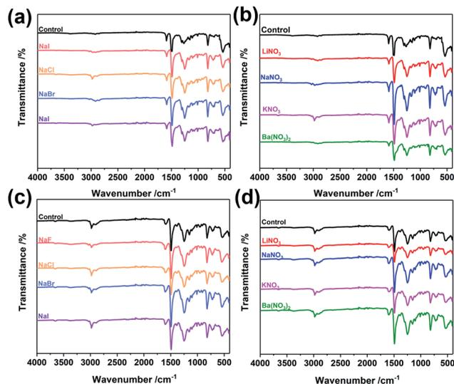
Fig. 1 FTIR spectra of PTPA: (a and b), before and after tuning by BXJ-Na salts; and PAPA: (c and d), before and after tuning by BXJ-NO<sub>3</sub> salts.
