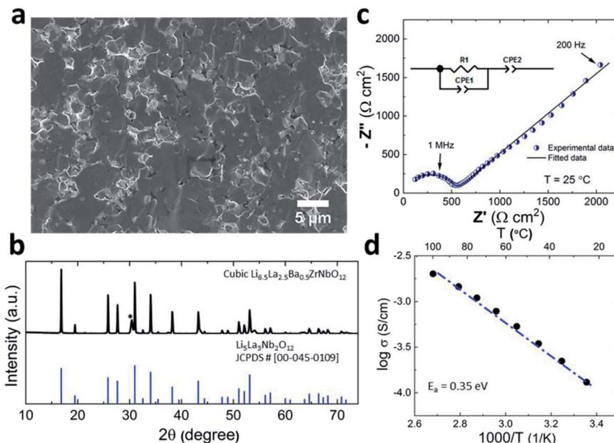
Fig. 1 (a) Cross-sectional SEM image of the LLZO SE. (b) XRD pattern for the synthesized LLZO compound confirming the formation of a cubic phase. \* Indicates the  $\text{BaZrO}_3$  impurity phase (c) Nyquist plot for LLZO SE at room temperature. (d) Arrhenius plot of the bulk conductivity of the LLZO SE over a temperature range of 25–100 °C.
