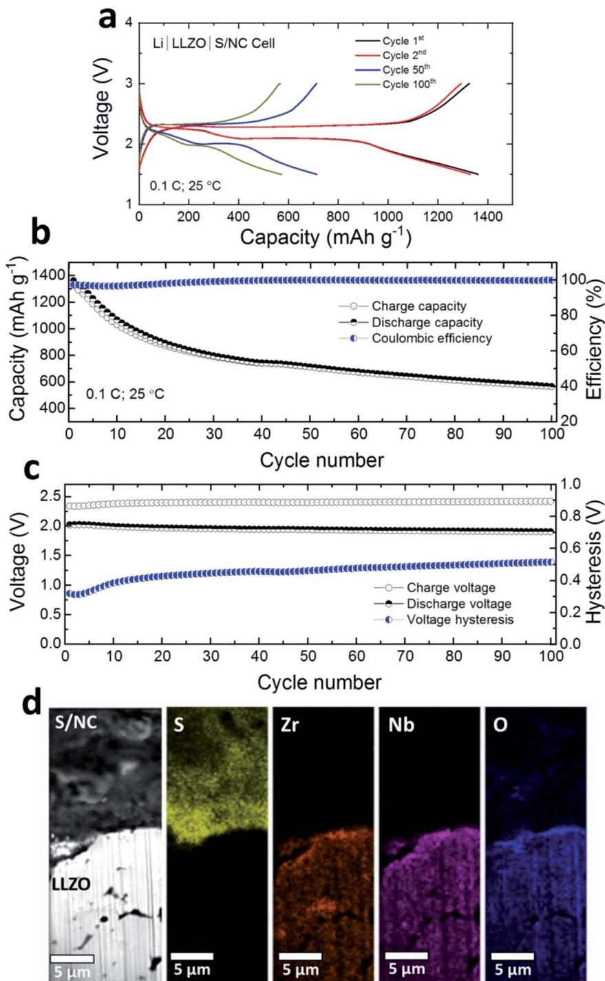
**Fig. 3** (a–c) Electrochemical performance of a Li|LLZO|S/NC cell tested at 0.1C-rate at 25 °C, (a) galvanostatic charge/discharge voltage profiles of the 1st, 2nd, 50th and 100th cycle, (b) cycle performance and coulombic efficiency, and (c) voltage hysteresis and average charge/discharge voltages of the cell from the 1st to 100th cycle. (d) Cross-sectional FIB-SEM image and elemental map of the interface between LLZO SE and the S/NC cathode of the cycled cell.
