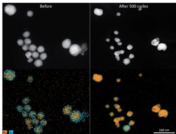
Fig. 6 Identical location TEM with STEM images and EDX mapping, before and after dealloying for 500 cycles in 1 M HClO<sub>4</sub>.
