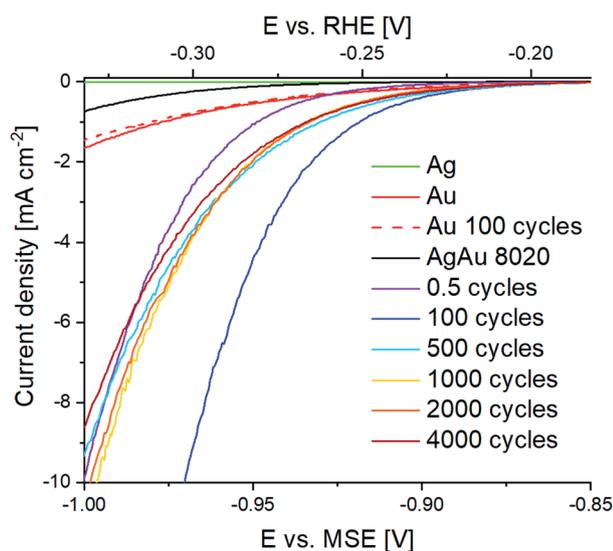
Fig. 8 Averaged catalytic LSV curves from multiple independent experiments at  $2 \text{ mV s}^{-1}$  in  $0.5 \text{ M H}_2\text{SO}_4$  using pure silver and pure gold; 100 cycles "dealloyed" gold, non-dealloyed  $\text{AgAu 80 : 20}$  and dealloyed  $\text{AgAu}$  nanoparticles after different numbers of dealloying cycles. The plotted currents are normalized to the electrochemically determined surface area of the nanoparticles.
