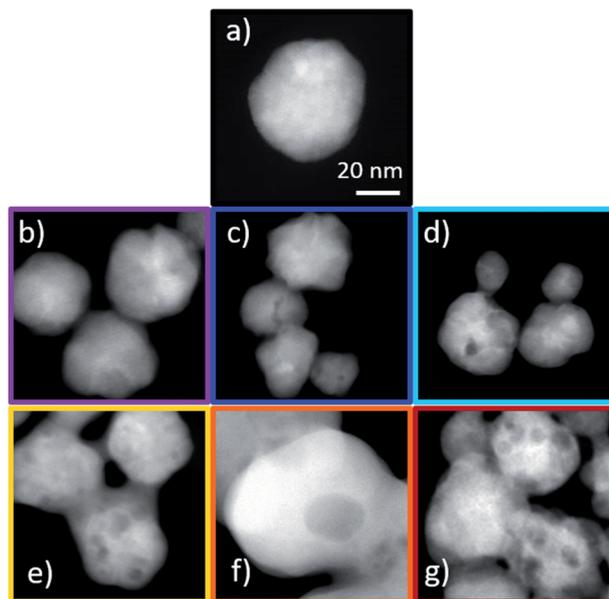
Fig. 7 Zoomed in STEM images from different samples of (a) untreated  $\text{Ag}_{80}\text{Au}_{20}$  nanoparticles, (b) after 0.5 cycles, (c) after 100 cycles, (d) after 500 cycles, (e) after 1000 cycles, (f) after 2000 cycles, and (g) after 4000 cycles, the scale bar is the same for all images.
