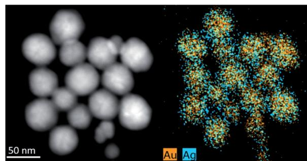
Fig. 1 STEM-HAADF image of untreated Ag<sub>80</sub>Au<sub>20</sub> nanoparticles (left), EDX elemental mapping of the nanoparticles (right) shows alloy nanoparticles with a Au-rich core.
