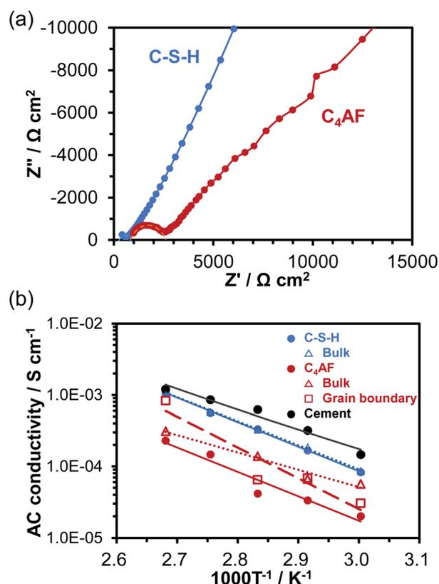
Fig. 4 (a) Impedance spectra of C-S-H and C<sub>4</sub>AF at 60 °C. (b) Temperature dependence of AC conductivity for C-S-H and C<sub>4</sub>AF.
