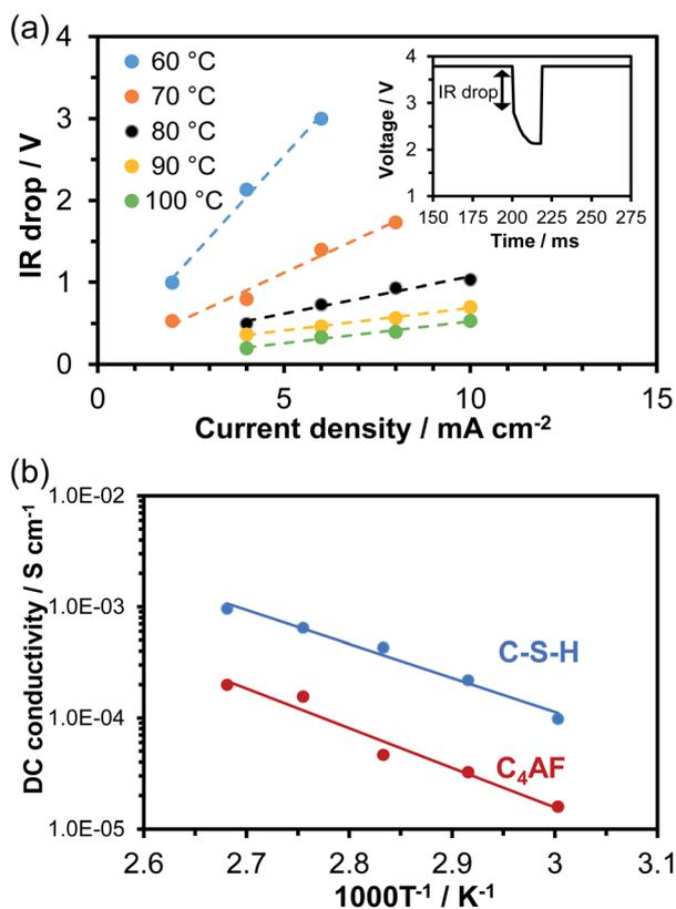
Fig. 3 (a)  $IR$  drop as a function of the current density recorded for C-S-H at various temperatures. The inset is the transient change in voltage within a current interruption period. (b) Temperature dependence of DC conductivity for C-S-H and C<sub>4</sub>AF.
