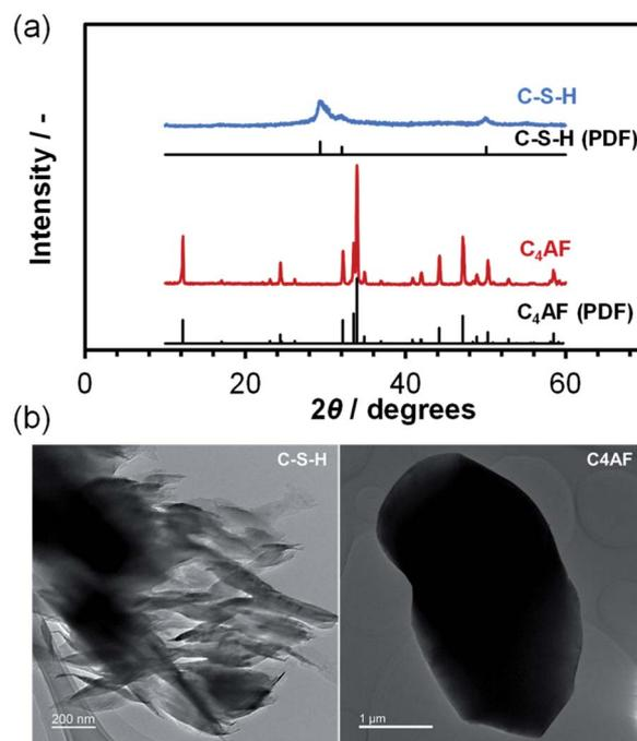
Fig. 1 (a) XRD patterns for C-S-H and C<sub>4</sub>AF. The PDFs of Ca<sub>1.5</sub>-SiO<sub>3.5</sub>·*x*H<sub>2</sub>O and Ca<sub>2</sub>FeAlO<sub>5</sub> are included for reference. (b) TEM images of C-S-H and C<sub>4</sub>AF.
