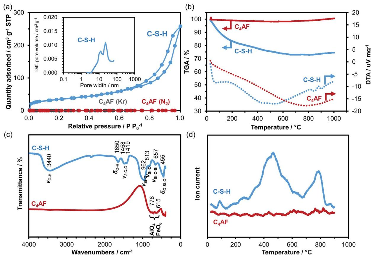
Fig. 2 (a) Adsorption/desorption isotherms of nitrogen for C-S-H and C<sub>4</sub>AF and of krypton for C<sub>4</sub>AF. The inset is the pore size distribution of C-S-H. (b) TG and DTA curves and (c) FTIR spectra of C-S-H and C<sub>4</sub>AF. (d) Desorption profiles of CO<sub>2</sub> for C-S-H and C<sub>4</sub>AF.
