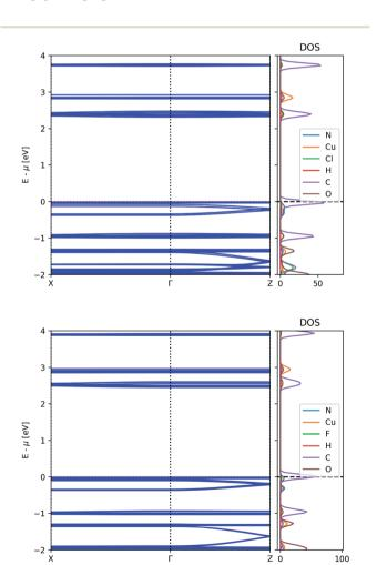
Fig. 6 Electronic band structure and atom-projected density of states of MOF-649 with CI (top) and F (bottom).
