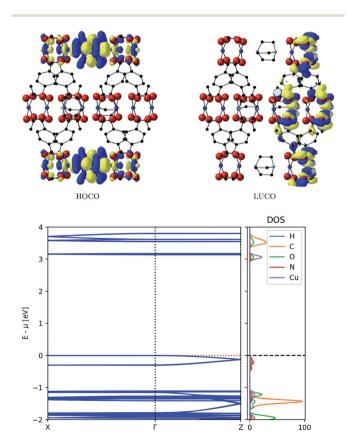
Fig. 3 Top: Frontier orbitals of DMOF-1. Bottom: Electronic band structure (left) and atom-projected density of states (right) of DMOF-1.
