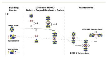
Fig. 5 Energy (Kohn–Sham eigenvalue) alignment of the buildingblock molecular orbitals that combine to form the crystal orbitals in the studied frameworks.
