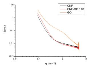
Fig. 6 Small angle X-ray scattering profiles (intensity (arbitrary units) versus scattering vector q ( $q = (2\pi/d)$ )) of CNF, CNF-GO 0.07 vol% and GO nanopaper films, where the X-ray beam is perpendicular to the film plane.
