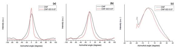
Fig. 5 Azimuthal angle distribution of CNF and CNF-GO 0.07 at three different q ranges. (a)  $q = 0.6 - 0.9 \text{ nm}^{-1}$ , (b)  $q = 1 - 2 \text{ nm}^{-1}$  and (c)  $q = 15 - 2 \text{ nm}^{-1}$ 18 nm<sup>-1</sup>.
