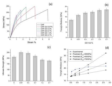
Fig. 3 Representative stress–strain curves of CNF–GO nanopaper films (a) Young's modulus (b) and ultimate strength (c) as a function of GO content. (d) Shows experimental Young's modulus of CNF–GO films *versus* GO content. Predicted modulus data are calculated from eqn (3) (rule of mixtures) assuming three different and very high values for GO modulus, the CNF phase is assumed to have a modulus  $E_2 = 13.5$  GPa, based on the present experimental data for CNF films.
