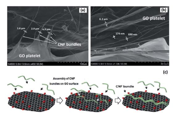
Fig. 7 FE-SEM images of freeze-dried CNF-GO 0.07 (a and b) and representation of suggested mechanism for assembly of CNF bundles on GO surface (c).
