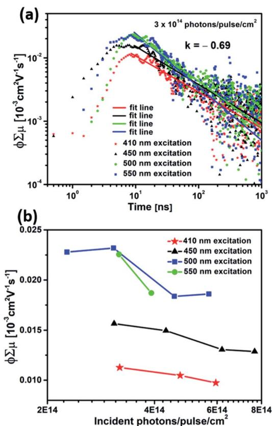
Fig. 4 (a) TRMC signal under various incident laser pulse intensities for a  $\text{Cu}_5\text{V}_2\text{O}_{10}$  film synthesized by spray pyrolysis on a quartz substrate at different wavelengths. (b) Maximum TRMC signal  $(\phi \sum \mu)_{\text{max}}$  vs. incident laser pulse intensity for  $\text{Cu}_5\text{V}_2\text{O}_{10}$  films deposited on quartz substrates under different laser wavelengths.
