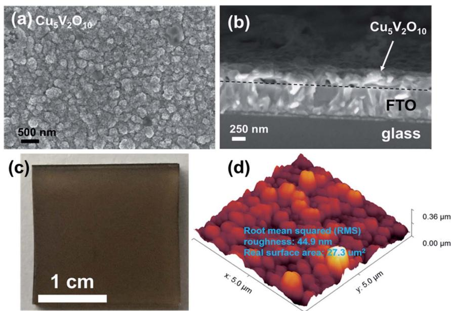
Fig. 2 (a) Top-view and (b) cross-section SEM images of a  $\text{Cu}_5\text{V}_2\text{O}_{10}$  thin film deposited on FTO annealed at 550 °C in air for 4 hours. (c) Photograph of a  $\text{Cu}_5\text{V}_2\text{O}_{10}$  thin film deposited on an FTO-coated glass substrate. (d) Atomic force microscopy (AFM) image of a ~250 nm  $\text{Cu}_5\text{V}_2\text{O}_{10}$  film deposited on an FTO substrate.
