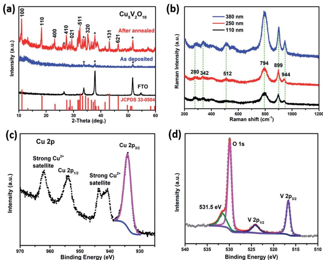
Fig. 1 (a) XRD diffractogram for a  $\text{Cu}_5\text{V}_2\text{O}_{10}$  photocathode synthesized by spray pyrolysis on an FTO substrate. Red vertical lines represent the reference pattern for  $\text{Cu}_5\text{V}_2\text{O}_{10}$  photoelectrode (PDF no. 33-0504) (b) Raman spectra of the  $\text{Cu}_5\text{V}_2\text{O}_{10}$  films (annealed at 550 °C for 4 hours in air) with different thicknesses. XPS spectra of (c) Cu 2p, (d) V 2p and O 1s for  $\text{Cu}_5\text{V}_2\text{O}_{10}$  film.
