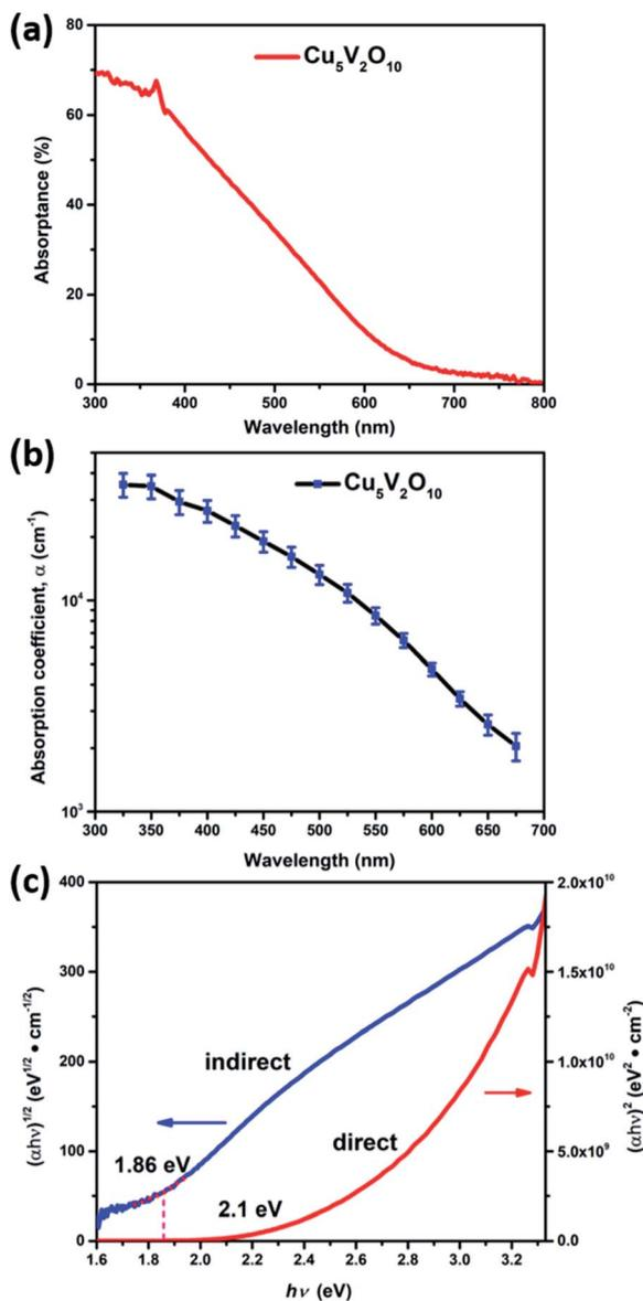
Fig. 3 (a) Absorbance spectra and (b) absorption coefficient for 250 nm thick  $\text{Cu}_5\text{V}_2\text{O}_{10}$  film deposited on quartz substrate. (c) Tauc plots for bandgap analysis of the  $\text{Cu}_5\text{V}_2\text{O}_{10}$  film. The indirect and direct bandgaps are estimated from inflection point and the intercept of the  $(\alpha h\nu)^{0.5}$  and  $(\alpha h\nu)^2$  curves with the  $x$ -axis, respectively.
