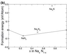
Fig. 5 (a) Formation energy per atom vs. sodium concentration in Na–Sn compounds calculated with the PBE (black) and HSE06 (red) functionals. (b) Formation energy per atom vs. sodium concentration in Na–N compounds calculated with the HSE06 functional. In both panels, the convex hull (black and red lines) are constructed by joining the lowest energy point structures obtained by the searches.
