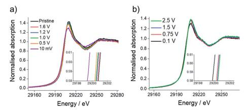
Fig. 8 Sn K-edge XANES spectra during: (a) first reduction and (b) first oxidation of microcrystalline  $Sn_3N_4$  as a function of cell potential. The insets show the central part of the absorption edge, magnified for clarity.
