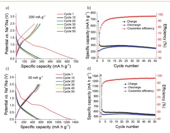
Fig. 3 Galvanostatic cycling (a and c) and plot of specific capacity vs. cycle number (b and d) of microcrystalline  $Sn_3N_4$  in Na half-cells at 200 mA  $g^{-1}$  (a and b) and 50 mA  $g^{-1}$  (c and d).
