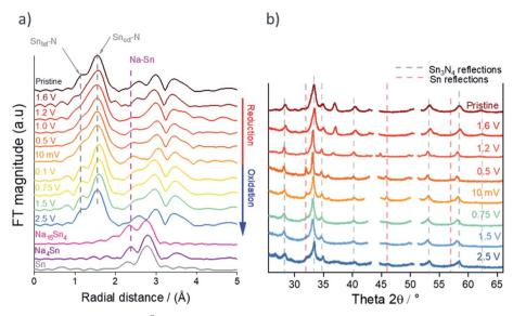
Fig. 9 (a) Magnitude of the Fourier transforms of  $K^3$ -weighted Sn K-edge EXAFS during initial reduction and oxidation of microcrystalline Sn<sub>3</sub>N<sub>4</sub>. The data of Na<sub>15</sub>Sn<sub>4</sub>, Na<sub>4</sub>Sn and Sn from the ICSD database is also included for comparison. (b) Corresponding ex situ XRD patterns, with peaks due to the Cu current collector omitted from the pattern.
