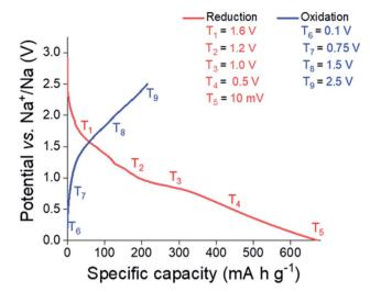
Fig. 7 Initial galvanostatic cycle of microcrystalline  $\rm Sn_3N_4$  depicting where samples were taken for the *ex situ* XRD, XANES and EXAFS studies.
