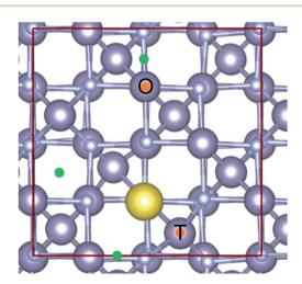
Fig. 6 A ball and stick representation of the Sn<sub>3</sub>N<sub>4</sub> structure. The large purple spheres are Sn; the smaller purple spheres are nitrogen. The Na interstitial in its lowest energy configuration is shown as a yellow sphere. Other sites considered are shown with green dots. The two substitutional sites for the substitution of Sn by Na are highlighted with orange dots (upper: octahedral, lower: tetrahedral). The unit cell is highlighted in red
