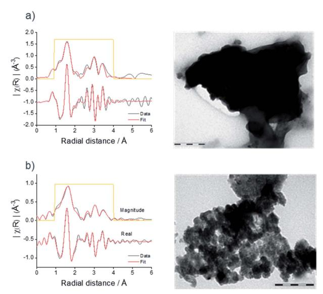
Fig. 2 Magnitude and real part of the Fourier transforms of  $K^3$ -weighted Sn K-edge EXAFS and TEM images of microcrystalline (a) and nanocrystalline (b) Sn<sub>3</sub>N<sub>4</sub>. The scale bar in (a) is 200 nm and in (b) it is 100 nm
