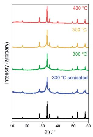
Fig. 1 Powder XRD patterns for the products of solvothermal synthesis at various temperatures. The black pattern denotes the literature  $Sn_3N_4$  reflection positions and intensities.<sup>75</sup>
