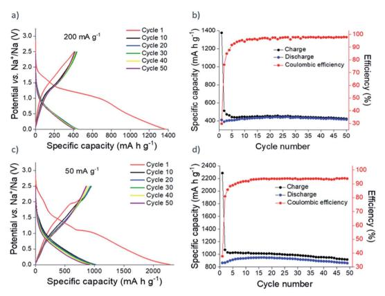
Fig. 4 Galvanostatic cycling (a and c) and plot of specific capacity vs. cycle number (b and d) of nanocrystalline Sn<sub>3</sub>N<sub>4</sub> in Na half-cells at 200 mA  $g^{-1}$  (a and b) and 50 mA  $g^{-1}$  (c and d).
