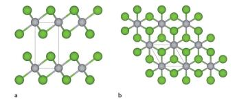
Fig. 1 (a) Side and (b) top views of the thermodynamically most stable TiSe<sub>2</sub> crystal structure under ambient conditions. The unit cell is represented by the solid black lines. Gray and green colours are reserved for Ti and Se ions, respectively.
