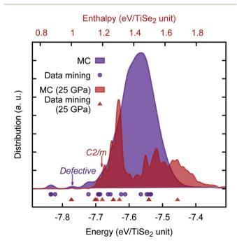
Fig. 6 Density distribution (with a Gaussian smearing of  $\sigma = 0.01 \, \text{eV}$ ) of the PSM IP energies from the KLMC-generated TiSe<sub>2</sub> structures. In this plot, purple and red are reserved for 0 and 25 GPa results. The calculated energies from the data mining procedure are shown as comparison below the curves
