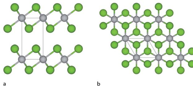
Fig. 1 (a) Side and (b) top views of the thermodynamically most stable  $\text{TiSe}_2$  crystal structure under ambient conditions. The unit cell is represented by the solid black lines. Gray and green colours are reserved for Ti and Se ions, respectively.
