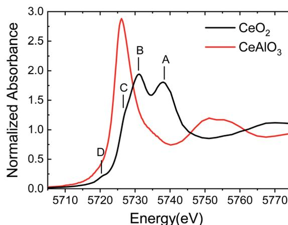
Fig. 2 Normalized Ce L<sub>3</sub> edge XANES spectra of the bulk regions of CeO<sub>2</sub> and CeAlO<sub>3</sub> films (as indicated), collected under ambient temperature and pressure.
