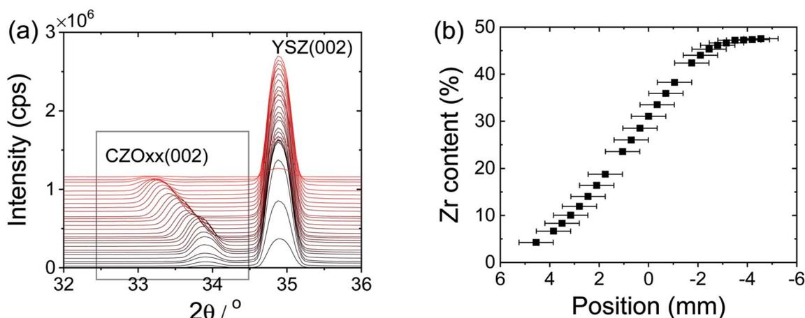
Fig. 1 X-ray diffraction study of graded ceria-zirconia film deposited on YSZ (001): (a) specular  $\theta$ - $2\theta$  scan, zoomed in to the region in the vicinity of the (002) peak; and (b) composition inferred from the refined lattice parameter.
