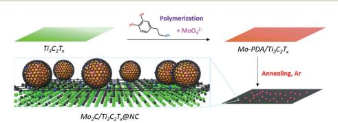
Fig. 1 Synthetic illustration of the preparation of Mo<sub>2</sub>C/Ti<sub>3</sub>C<sub>2</sub>T<sub>x</sub>@NC.
