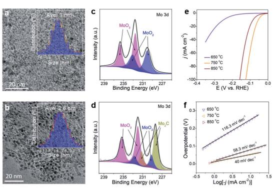
Fig. 5 TEM images of (a) M-650 and (b) M-850. The inset gives the size distributions of nanoparticles in the samples. High-resolution XPS Mo 3d spectra of (c) M-650 and (d) M-850. Polarization curves (e) and Tafel plots (f) of M-650, M-750, and M-850.
