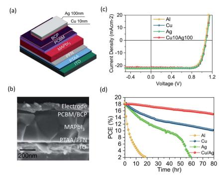
Fig. 1 (a) Schematic diagram of the typical device architecture investigated, here with the Cu-Ag bilayer electrode, (b) cross-section SEM image of a typical device, (c) J-V characteristics of devices with different electrodes as indicated, (d) stability measurements (PCE) of devices aged under continuous LED illumination in ambient air.
