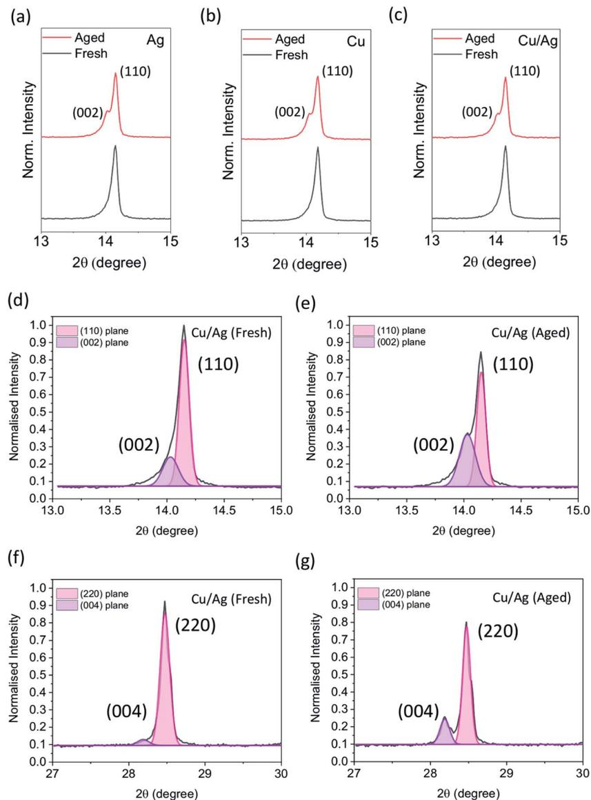
Fig. 5 XRD patterns of MAPbI<sub>3</sub> of devices with (a) Ag (b) Cu (c) Cu–Ag counter electrode before and after ageing under same condition in Fig. 1d. (d–g) The fitting plots of XRD data of MAPbI<sub>3</sub> before and after ageing.
