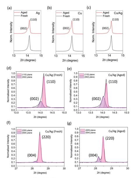
Fig. 5 XRD patterns of MAPbl<sub>3</sub> of devices with (a) Ag (b) Cu (c) Cu-Ag counter electrode before and after ageing under same condition in Fig. 1d. (d-g) The fitting plots of XRD data of MAPbl<sub>3</sub> before and after ageing.
