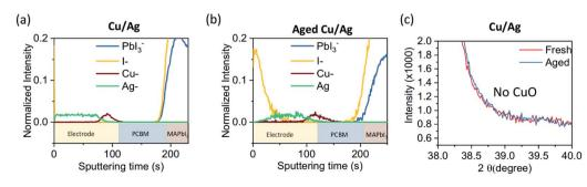
Fig. 3 Time-of-flight secondary ion mass spectrometry (ToF-SIMS) depth profile of device with (a) Cu-Ag (b) aged Cu-Ag electrode. (c) XRD spectra of Cu-Aq electrode on device before and after ageing. The devices are aged under same condition as Fig. 1d.
