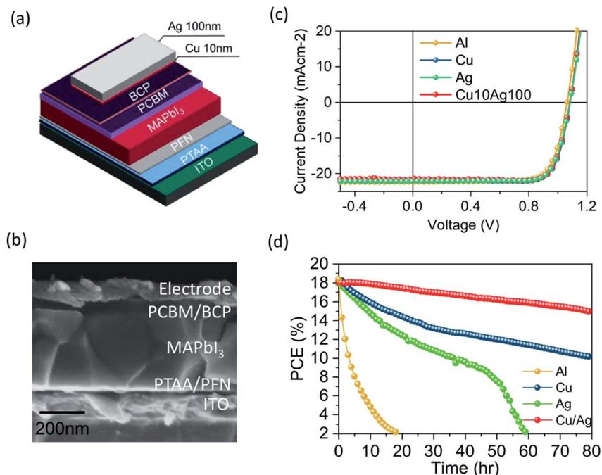
Fig. 1 (a) Schematic diagram of the typical device architecture investigated, here with the Cu–Ag bilayer electrode, (b) cross-section SEM image of a typical device, (c)  $J$ – $V$  characteristics of devices with different electrodes as indicated, (d) stability measurements (PCE) of devices aged under continuous LED illumination in ambient air.
