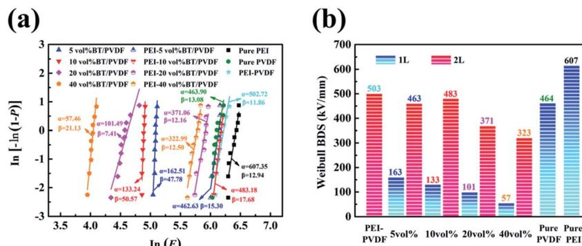
Fig. 4 (a) Weibull distribution plots and (b) characteristic breakdown strengths of the single layer and bilayer composites with different BaTiO<sub>3</sub> loading fractions.
