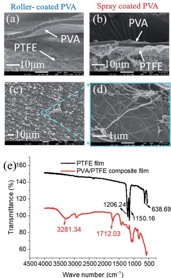
**Fig. 3** SEM micrographs of (a) roller coated and (b) spray coated PVA/PTFE composites where delamination of PVA is prevalent in the composites produced from roller coating. (c and d) The bottom surface of PVA selective layers was intertwined with PTFE fibers, indicating excellent compatibility between these materials. (e) The presence of spray coated PVA on PTFE supports was validated with FTIR analysis.
