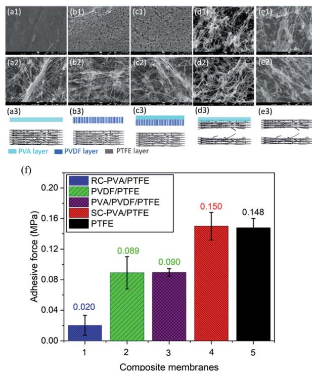
**Fig. 4** SEM images of the bottom surface from the top layer and the upper surface of the support layer, and a schematic diagram showing the tearing locations of the RC-PVA/PTFE (a1–a3), PVDF/PTFE (b1–b3), PVA/PVDF/PTFE (c1–c3), SC-PVA/PTFE (d1–d3) and PTFE (e1–e3) membranes. (f) The adhesion strength between PVA dense selective layers and PTFE supports in the composites produced from roller coating and spray coating.
