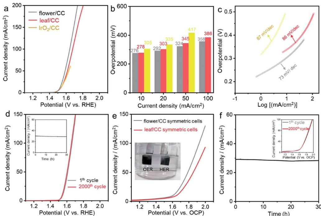
Fig. 4 The comparison of (a) LSVs, (b) overpotentials, (c) Tafel slopes and (d) stability tests for three nanomaterials in OER in O<sub>2</sub>-saturated 1.0 M KOH aqueous solution; (e) LSV and (f) stability test of the symmetric cells in the overall water splitting reaction. The scan rate is 5 mV s<sup>-1</sup>, and post-*iR* compensation is applied.
