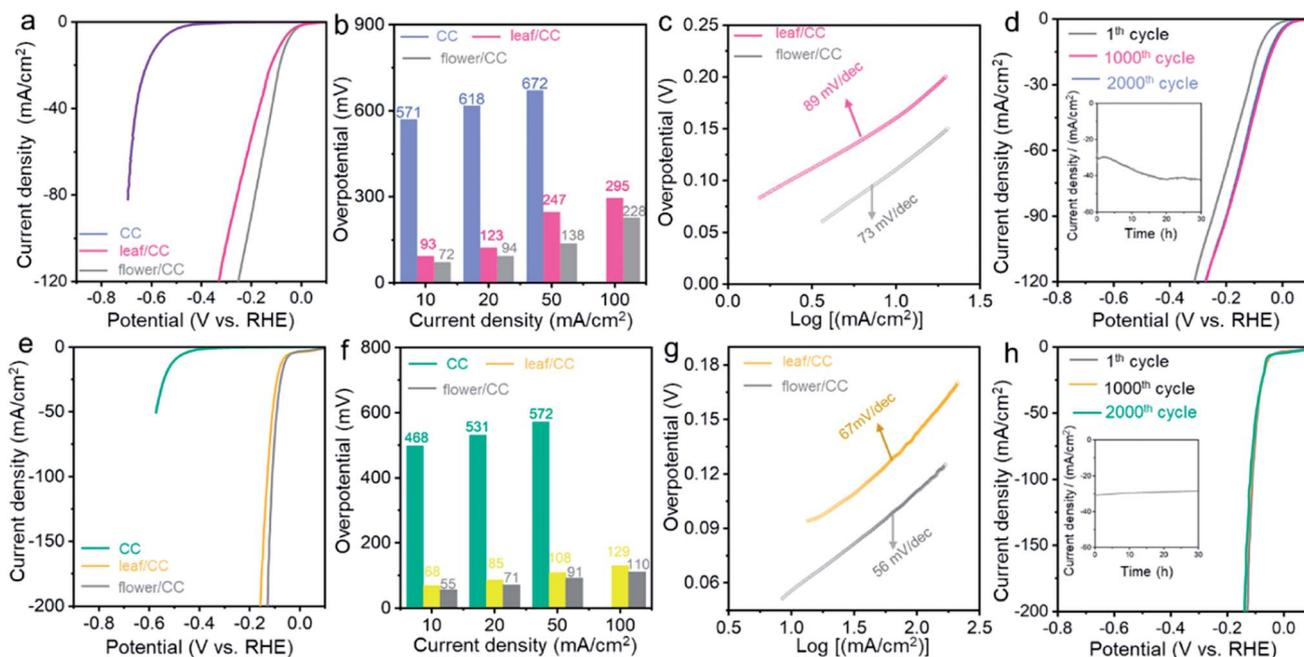
Fig. 3 The comparison of (a) LSVs, (b) overpotentials, (c) Tafel slopes and (d) stability tests for two nanomaterials in HER under neutral conditions with  $\text{H}_2$ -saturated phosphate buffer solution. The comparison of (e) LSVs, (f) overpotentials, (g) Tafel slopes and (h) stability tests for two nanomaterials in HER in  $\text{H}_2$ -saturated  $1.0 \text{ M KOH}$  aqueous solution. The scan rate is  $5 \text{ mV s}^{-1}$ , and post-*iR* compensation is applied.
