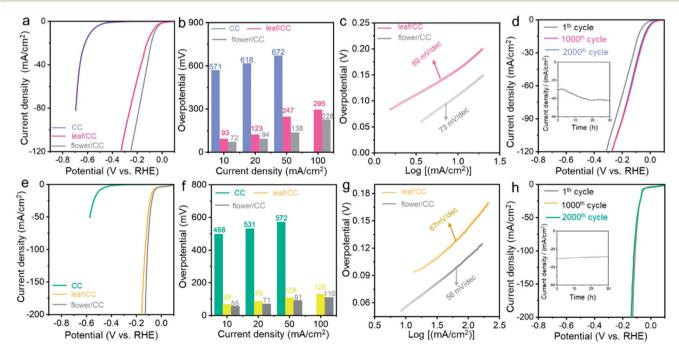
Fig. 3 The comparison of (a) LSVs, (b) overpotentials, (c) Tafel slopes and (d) stability tests for two nanomaterials in HER under neutral conditions with H<sub>2</sub>-saturated phosphate buffer solution. The comparison of (e) LSVs, (f) overpotentials, (g) Tafel slopes and (h) stability tests for two nanomaterials in HER in  $H_2$ -saturated 1.0 M KOH aqueous solution. The scan rate is 5 mV s<sup>-1</sup>, and post-iR compensation is applied
