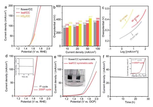
Fig. 4 The comparison of (a) LSVs, (b) overpotentials, (c) Tafel slopes and (d) stability tests for three nanomaterials in OER in  $O_2$ -saturated 1.0 M KOH aqueous solution; (e) LSV and (f) stability test of the symmetric cells in the overall water splitting reaction. The scan rate is 5 mV s<sup>-1</sup>, and post-iR compensation is applied.
