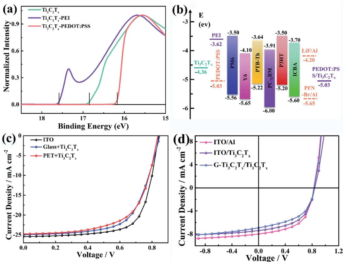
Fig. 3 OPVs performance using MXene transparent electrodes. (a) Ultraviolet photoelectron spectroscopy (UPS) secondary electron cut-off region of Ti<sub>3</sub>C<sub>2</sub>T<sub>x</sub> and Ti<sub>3</sub>C<sub>2</sub>T<sub>x</sub> electrodes modified by PEDOT:PSS and PEI. (b) Energy level diagram of OPV devices. (c) *J*-*V* curves of OPV devices based on PM6:Y6 with different electrodes. (d) *J*-*V* curves of OPV devices based on P3HT:ICBA with different electrodes.
