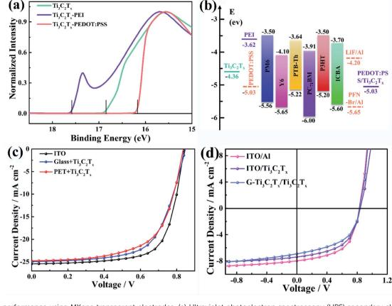
Fig. 3 OPVs performance using MXene transparent electrodes. (a) Ultraviolet photoelectron spectroscopy (UPS) secondary electron cut-off region of  $Ti_3C_2T_x$  and  $Ti_3C_2T_x$  electrodes modified by PEDOT:PSS and PEI. (b) Energy level diagram of OPV devices. (c) J-V curves of OPV devices based on PM6:Y6 with different electrodes. (d) J-V curves of OPV devices based on P3HT:ICBA with different electrodes.
