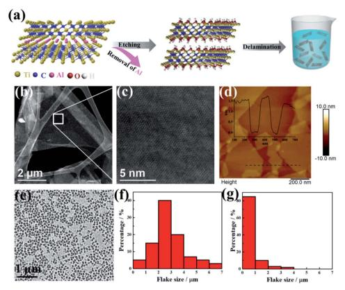
Fig. 1 Fabrication of the  $Ti_3C_2T_x$  MXene colloidal solution. (a) The MXene prepared from the  $Ti_3AlC_2$  precursor using the MILD method. (b) Lowmagnification and (c) high-magnification scanning transmission electron microscopy of single  $Ti_3C_2T_x$  sheets dispersed onto a lacy carbon grid. (d) AFM image of a  $Ti_3C_2T_x$  single layer. (e) Top view SEM image of small sized  $Ti_3C_2T_x$ . The  $Ti_3C_2T_x$  flake size distributions before (f) and after (g) sonication
