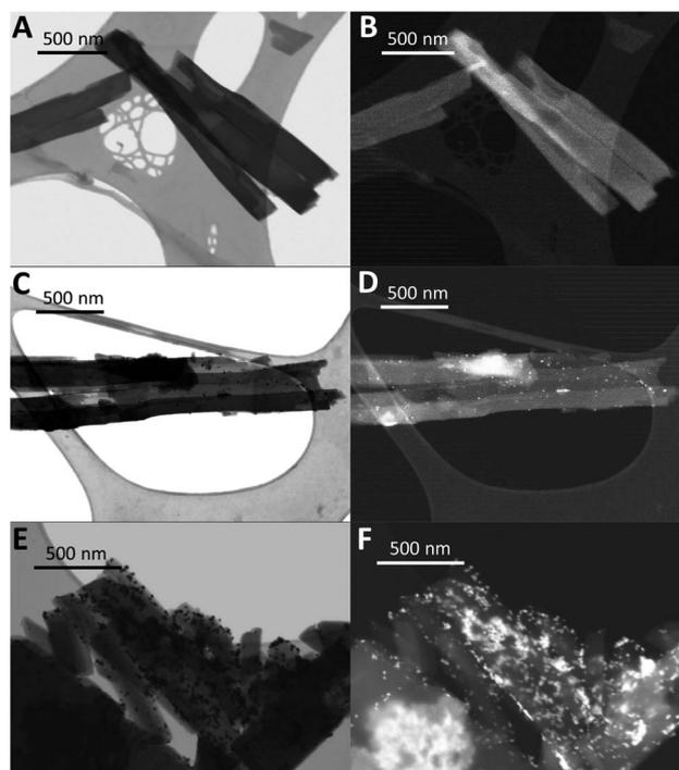
Fig. 5 STEM images of **TBAP- $\alpha$**  in (A) BF mode and (B) HADF mode, with 1 wt% photodeposited Pt in (C) BF mode and (D) HADF mode and with 4 wt% photodeposited Pt in (E) BF mode and (F) HADF mode.
