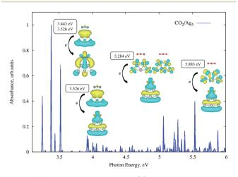
Fig. 6 UV-Vis absorption spectra for  $CO_2$  physisorbed on unsupported  $Cu_5$  clusters, as obtained at the TDDFT level with the PBE-D3(BJ) scheme. The orbitals responsible of the most relevant transitions involving electron transfer from the  $Cu_5$  cluster to the physisorbed  $CO_2$  molecule are also shown. The insets present density isosurfaces of these orbitals. A cluster model has been used (see the Methods section).
