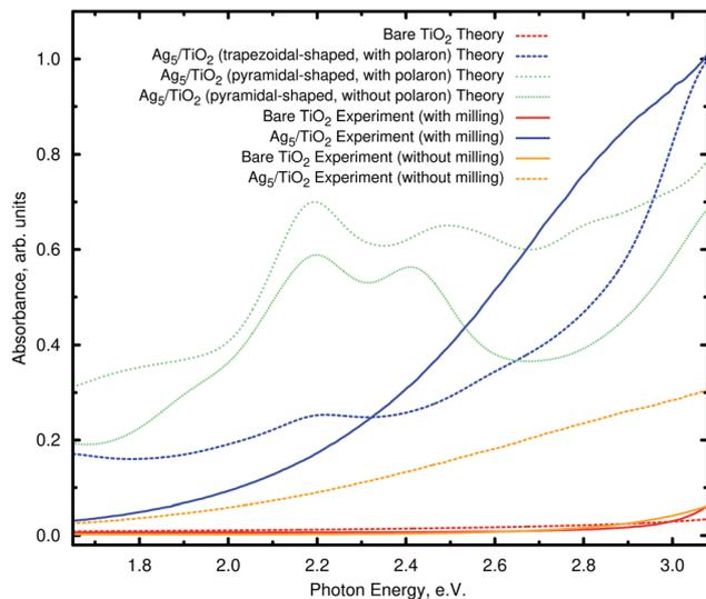
Fig. 5 Comparison of the theoretical and experimental absorbance in the visible region. The experimental absorbance  $A$  has been calculated via diffuse reflectance spectroscopy (DRS) measurements from the diffuse reflectance signal  $R_d$  as  $A = \log_{10}(1/R_d)$ . The units of absorbance are arbitrary units.
