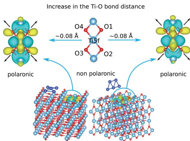
Fig. 1 Figure illustrating the formation of small polarons at fivefold coordinated titanium atoms ( $\text{Ti}_{5f}$ ) next to adsorbed  $\text{Ag}_5$  clusters, adopting both pyramidal- (left) and trapezoidal-shaped (right) structures.
