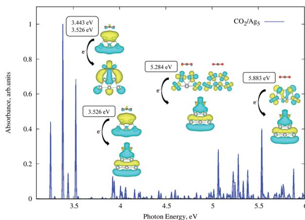
Fig. 6 UV-Vis absorption spectra for  $\text{CO}_2$  physisorbed on unsupported  $\text{Cu}_5$  clusters, as obtained at the TDDFT level with the PBE-D3(BJ) scheme. The orbitals responsible of the most relevant transitions involving electron transfer from the  $\text{Cu}_5$  cluster to the physisorbed  $\text{CO}_2$  molecule are also shown. The insets present density isosurfaces of these orbitals. A cluster model has been used (see the Methods section).
