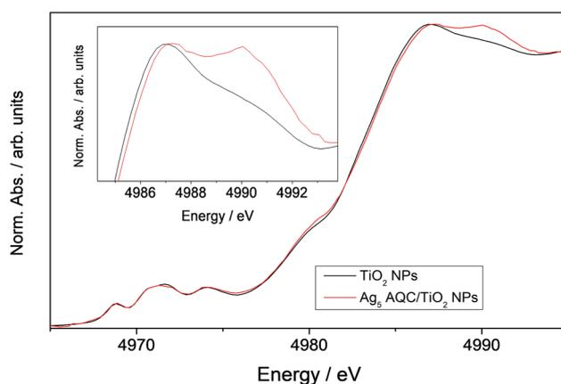
**Fig. 2** XANES spectra at the Ti K-edge of TiO<sub>2</sub> NPs (black line) and the Ag<sub>5</sub> atomic quantum cluster (AQC) supported on TiO<sub>2</sub> NPs (red line).
