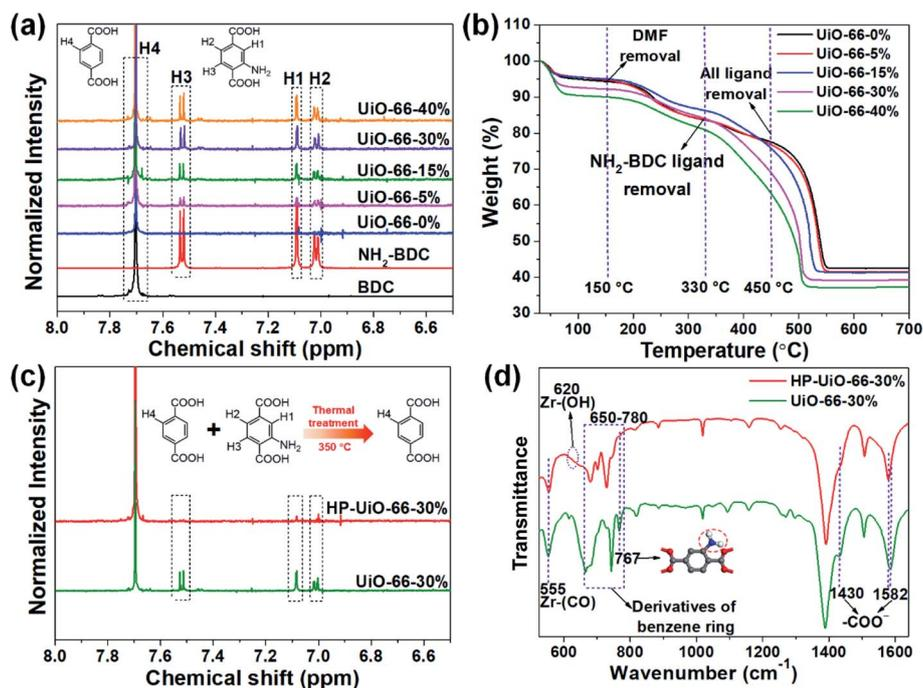
Fig. 2 (a) Dissolution/<sup>1</sup>H NMR spectra and (b) thermogravimetric analyses (TGA) of UiO-66-*X*% (*X* = 0, 5, 15, 30, and 40). (c) Dissolution/<sup>1</sup>H NMR spectra and (d) FT-IR spectra of UiO-66-30% and HP-UiO-66-30%.
