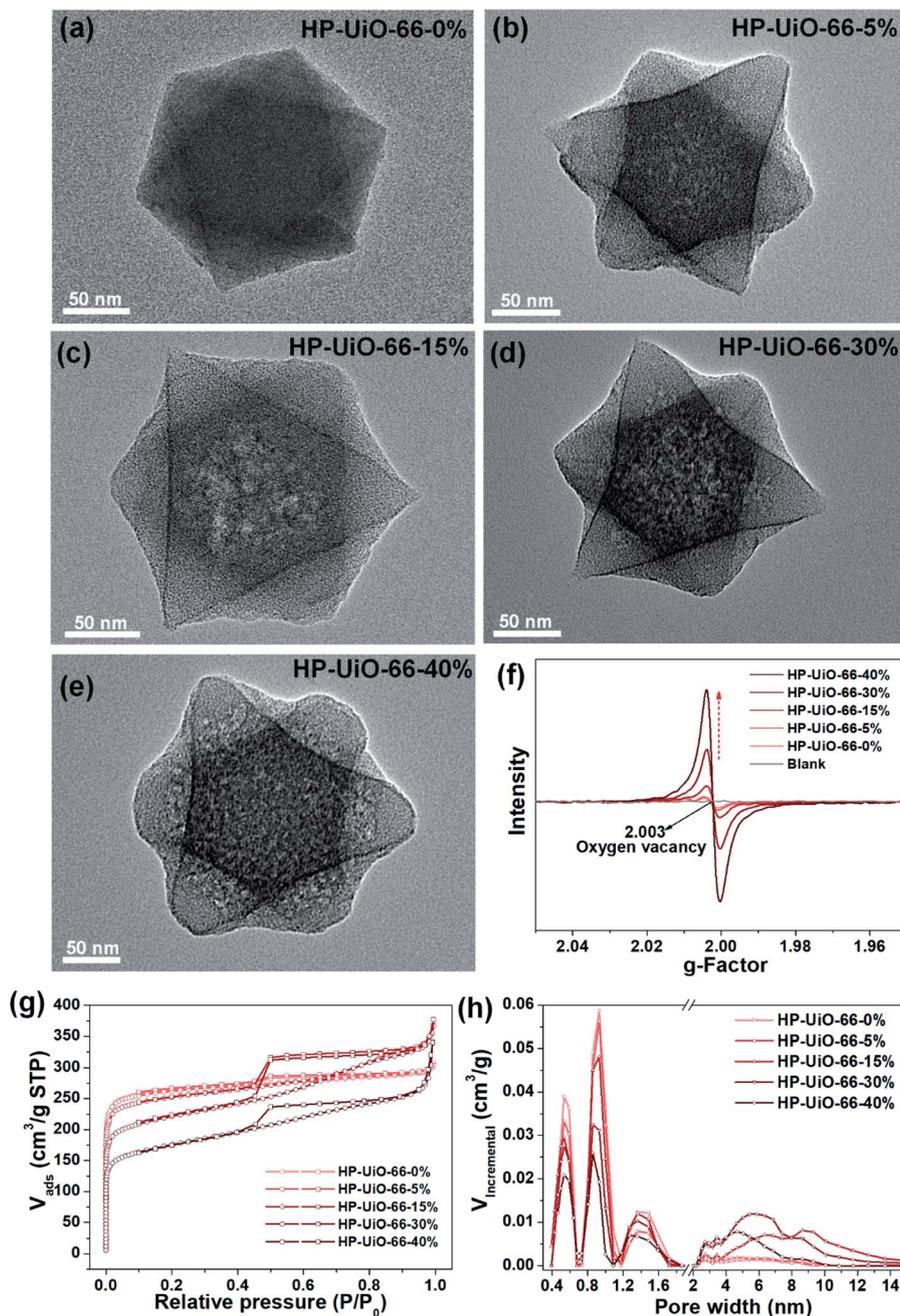
Fig. 1 (a–e) TEM images, (f) EPR spectra, (g)  $N_2$  adsorption/desorption isotherms, (h) pore size distributions based on density-functional theory (DFT) analysis of HP-UiO-66- $X\%$  ( $X = 0, 5, 15, 30, 40$ ).
