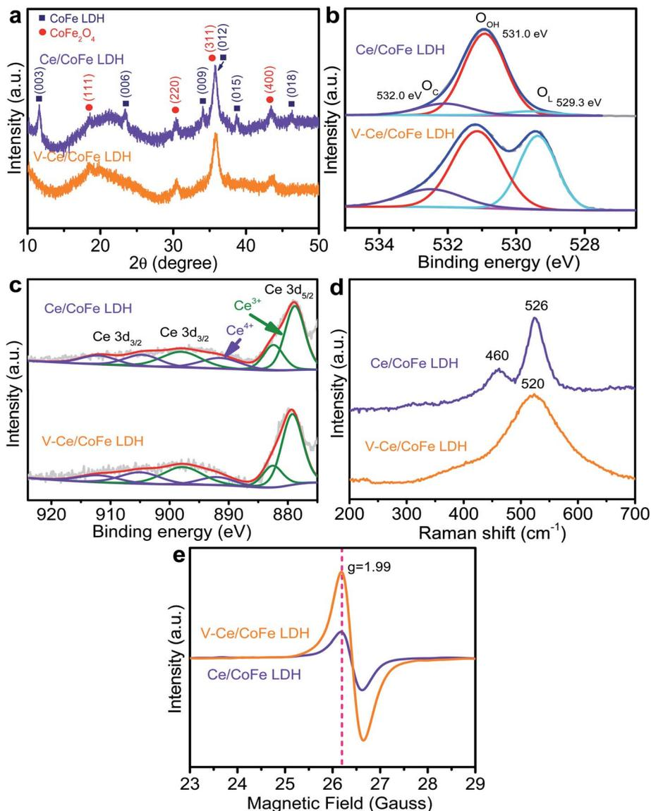
Fig. 3 (a) XRD patterns of Ce/CoFe LDH and V-Ce/CoFe LDH powders; (b) O 1s and (c) Ce 3d XPS spectra, (d) Raman spectra, and (e) EPR results of Ce/CoFe LDH and V-Ce/CoFe LDH.
