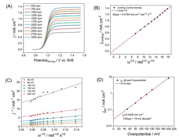
Fig. 1 (A) Linear-sweep voltammetry at a scan rate of 5 mV s<sup>-1</sup> with the RDE (glassy carbon) in freshly prepared 1 M H<sub>2</sub>SO<sub>4</sub> containing 1 mM BQDS. The rotation rate increased from 500 to 3000 rpm. (B) Levich plot of the square root of rotation rate vs. the limiting current for BQDS. (C) Koutecký-Levich plot for different overpotentials. (D) Tafel logarithmic plot of overpotential vs. kinetic current density.
