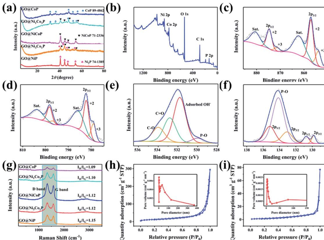
Fig. 3 (a) The XRD patterns, the XPS spectra of (b) the survey, (c) Ni 2p, (d) Co 2p, (e) O 1s and (f) P 2p for GO@NiCoP, (g) the Raman spectra, the  $\text{N}_2$  adsorption–desorption isotherms and pore-size distribution (inset) of (h) GO@NiCoP and (i) NiCoP.
