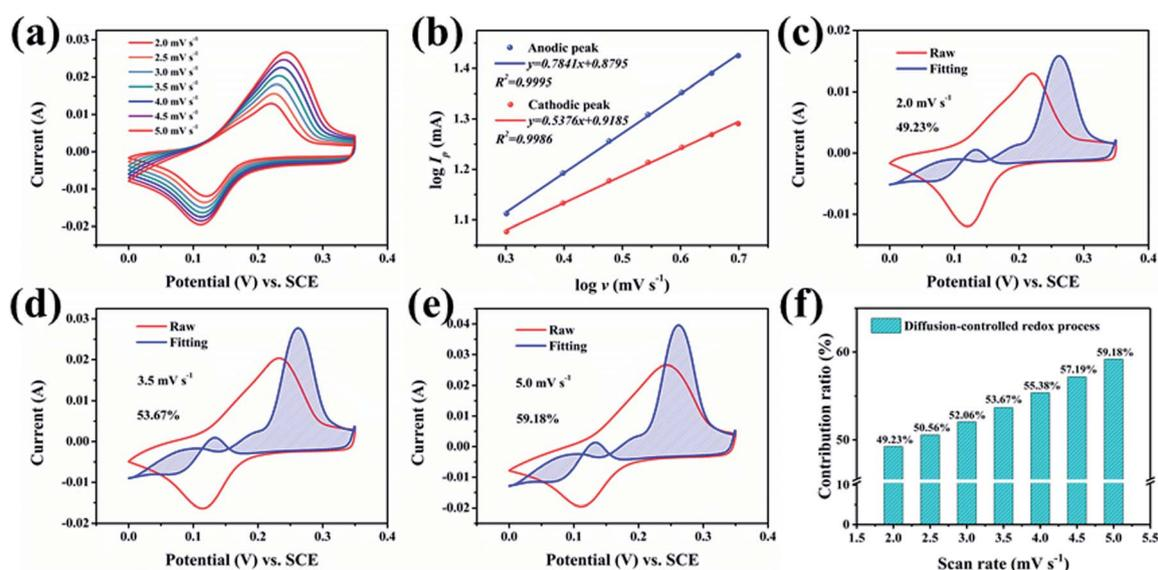
Fig. 5 (a) The CV curves of GO@NiCoP at low scan rates, (b) the plot of  $\log I_p$  *versus*  $\log \nu$  for the GO@NiCoP electrode at low scan rates, (c–e) separation of the capacitive and diffusion currents in the GO@NiCoP electrode at a scan rate of 2.5, 3.5 and 5.0 mV s<sup>–1</sup>, respectively, (f) the capacitance ratio of the surface capacitance effect at different scan rates.
