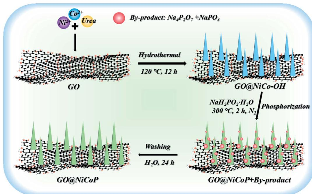
Scheme 1 The schematic illustration for the preparation process of GO@NiCoP.
