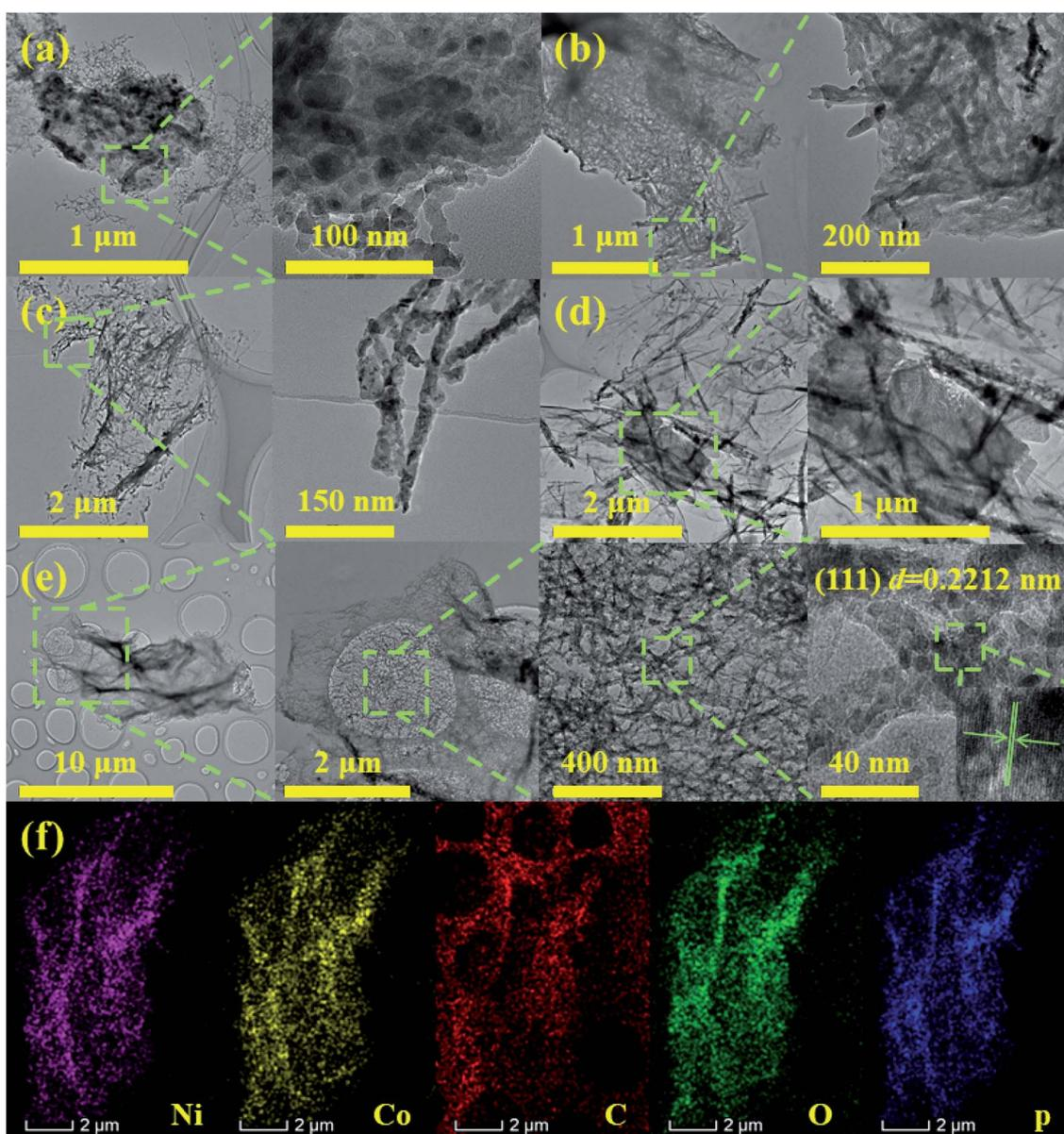
Fig. 2 The TEM images of (a) GO@NiP, (b) GO@Ni<sub>3</sub>Co<sub>1</sub>P, (c) GO@Ni<sub>1</sub>Co<sub>3</sub>P, (d) GO@CoP, (e) GO@NiCoP, (f) the elemental distribution sum spectra.
