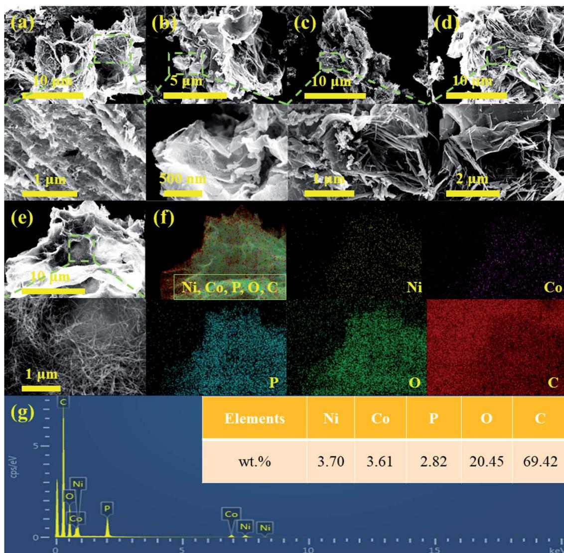
Fig. 1 The SEM images of (a) GO@NiP, (b) GO@Ni<sub>3</sub>Co<sub>1</sub>P, (c) GO@Ni<sub>1</sub>Co<sub>3</sub>P, (d) GO@CoP, (e) GO@NiCoP, (f) the elemental distribution sum spectra and (g) the corresponding EDS mapping of GO@NiCoP.
