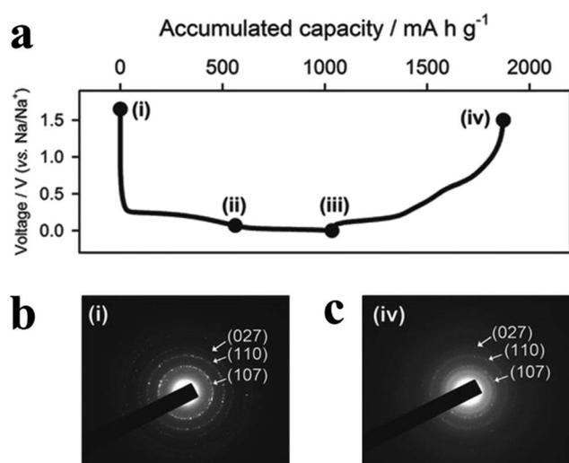
Fig. 17 (a) First galvanostatic charge and discharge profiles of the  $\text{Sn}_4\text{P}_3$  electrode obtained without an FEC additive. The different points indicate (i) pristine, (ii) 0.07 V, (iii) 0 V and (iv) 1.5 V. (b, c) Electron diffraction (ED) patterns at the points (i) and (iv) in (a), respectively. Reproduced with permission.<sup>77</sup> Copyright 2014, WILEY-VCH.
