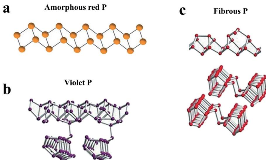
Fig. 2 Characteristic structural fragments of (a) amorphous RP; (b) violet P (Hittorf's P); (c) fibrous P. (a) Reproduced with permission.<sup>100</sup> Copyright 2019, WILEY-VCH. (b, c) Reproduced with permission.<sup>113</sup> Copyright 2017, Wiley-VCH.
