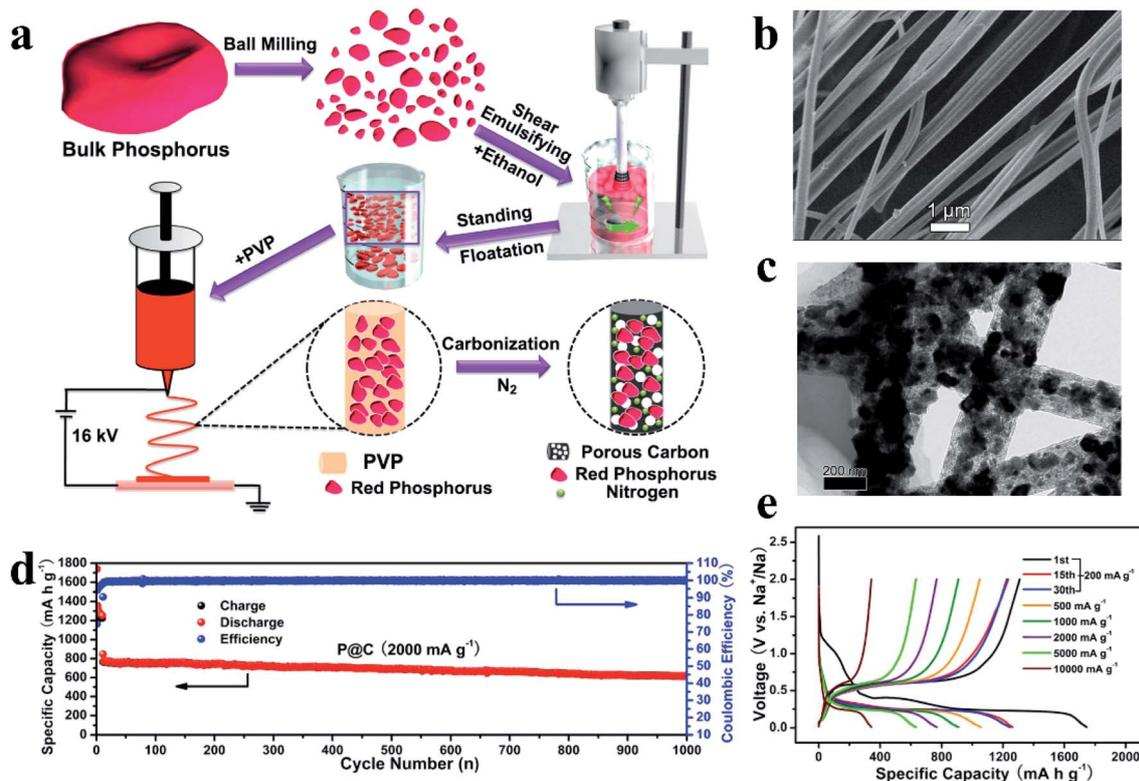
Fig. 5 (a) Schematic illustration of the preparation process for RP@C nanofibers. (b, c) SEM and TEM images of red P@C nanofibers. (d) Long-term cycling stability of the P@C electrode at a current density of  $2000 \text{ mA g}^{-1}$ . (e) Charge/discharge profiles obtained at various rates of the P@C electrode in the voltage range of 0.01–2 V vs.  $\text{Na}^+/\text{Na}$ . Reproduced with permission.<sup>127</sup> Copyright 2017, Elsevier B.V.
