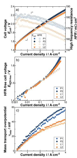
Fig. 3 (a) Polarization curves and area specific HFR. (b) Tafel-plot and corresponding (extrapolated) Tafel-lines. The Tafel-lines are fitted between 10 and 100 mA cm $^{-2}$ . (c) The difference between the HFR-free cell voltage and the extrapolated Tafel-lines, *i.e.* mass transport overpotentials.
