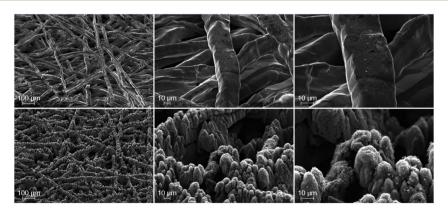
Fig. 1 SEM-images before PEMWE cell tests of the PTL surface, which is later in contact with the CL, of the pristine (top) and the laser-structured PTLs (bottom) each at magnifications of  $100 \times$ ,  $500 \times$  and  $1000 \times$ , from left to right.
