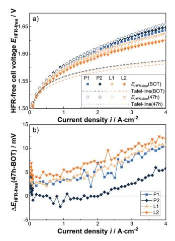
Fig. 5 (a) HFR-free cell voltage and extrapolated Tafel-lines at BOT and after the first 30 h period at 4 A cm $^{-2}$ , *i.e.* 47 h, and (b) the corresponding difference in HFR-free cell voltage.
