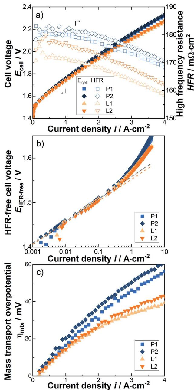
Fig. 3 (a) Polarization curves and area specific HFR. (b) Tafel-plot and corresponding (extrapolated) Tafel-lines. The Tafel-lines are fitted between 10 and 100  $\text{mA}\cdot\text{cm}^{-2}$ . (c) The difference between the HFR-free cell voltage and the extrapolated Tafel-lines, *i.e.* mass transport overpotentials.
