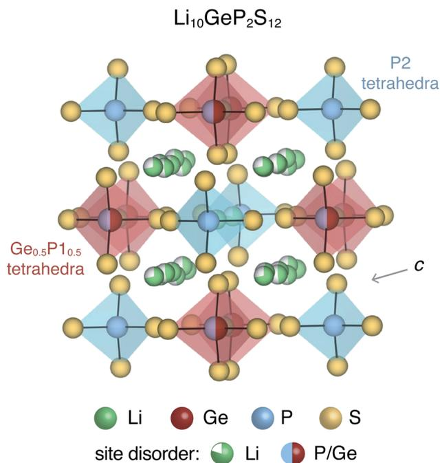
Fig. 1 Tetragonal crystal structure of  $\text{Li}_{10}\text{GeP}_2\text{S}_{12}$  contains  $\text{P}_2\text{S}_4$  tetrahedra and  $(\text{Ge}_{0.5}\text{P}_{1.0.5})\text{S}_4$  tetrahedra with partially occupied Li sites in the  $c$ -axis channels and in the  $a$ - $b$  plane bridging sites. The S sub-lattice and P2 sites are fully occupied.
