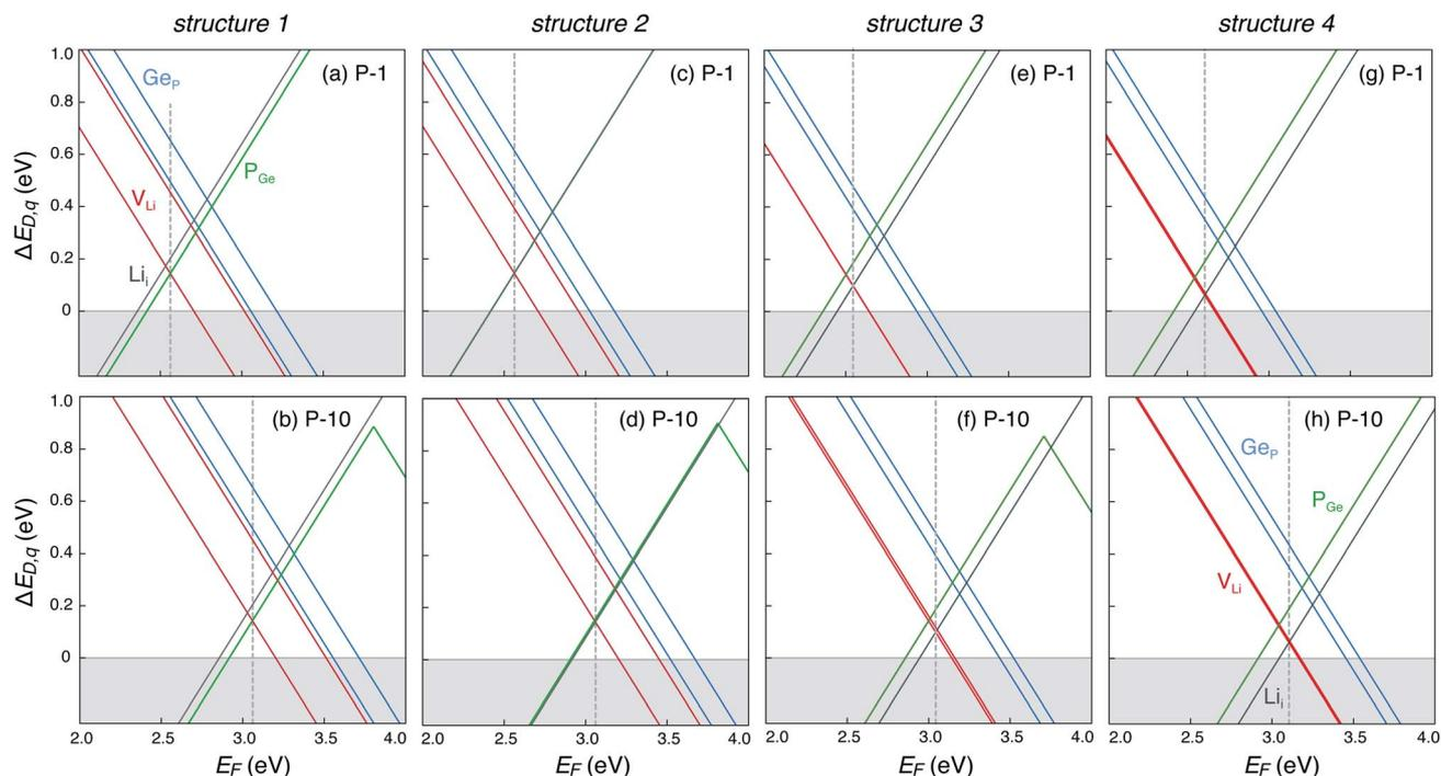
Fig. 5 Formation energies of native point defects ( $V_{Li}$ ,  $Li_i$ ,  $P_{Ge}$ , and  $Ge_P$ ) as functions of Fermi energy ( $E_F$ ) in LGPS structures 1–4 (Fig. 3) at elemental chemical potentials corresponding to P-1 (a, c, e and g), and P-10 (b, d, f and h).  $E_F$  is referenced to the valence band maximum. Multiple lines of the same color represent the same defect type at different Wyckoff sites.
