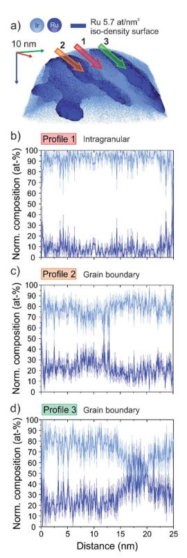
Fig. 3 APT composition profiles along intragranular and grain boundary regions within the bulk of an as-deposited sample. (a) 3D reconstruction of evaporated volume. Grain boundary regions are highlighted by means of Ru iso-density surfaces. (b) Intragranular composition profile exhibiting a more or less uniform composition within the bulk grains of the metallic alloy. (c and d) Grain boundary region composition profiles revealing a non-uniform Ru content along these interfaces
