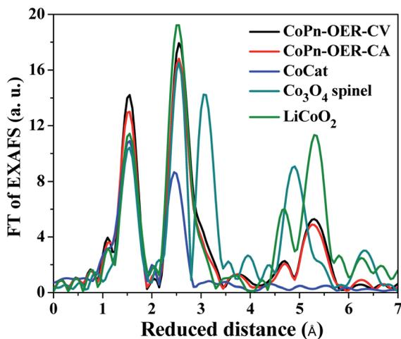
Fig. 6 FT of EXAFS of CoPn exposed to OER potentials compared with other catalysts. Two approaches to simulations are shown in Table S4.† Please note that  $\text{LiCoO}_2$  is isostructural to  $\text{CoOOH}$  resulting in indistinguishable EXAFS spectra.
