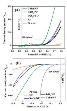
Fig. 2 (a) CV of OER and (b) LSV of HER for CoPn/NF and commercial noble metal-based catalysts in 1 M aqueous KOH at a scan rate of 1 mV
