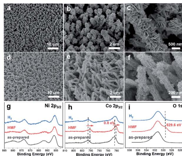
Fig. 6 SEM images of  $Cu_xS@Ni_{0.75}Co_{0.25}O_mH_n$  after catalyzing long-term HMF oxidation (a–c) and HER (d–f). Ni  $2p_{3/2}$  (g), Co  $2p_{3/2}$  (h) and O 1s (i) XPS spectra of  $Cu_xS@Ni_{0.75}Co_{0.25}O_mH_n$  after catalyzing long-term HMF oxidation (labeled as 'HMF') and hydrogen evolution reaction (labeled as ' $H_2$ ').
