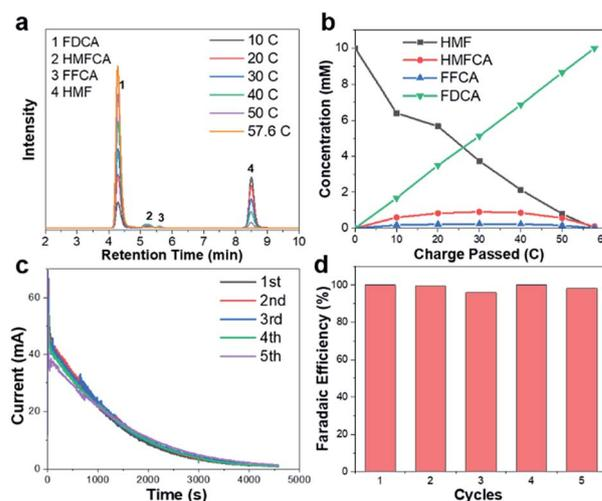
Fig. 3 (a) HPLC chromatogram traces of electrolyte during the electrochemical oxidation of HMF catalyzed by  $\text{Cu}_x\text{S}@Ni_{0.75}\text{Co}_{0.25}\text{O}_m\text{H}_n$  at 1.32 V vs. RHE. (b) Concentration profiles of oxidation products with increasing charge. (c) Current–time curves and (d) faradaic efficiency towards FDCA in 5 successive runs.
