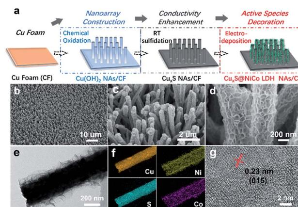
Fig. 1 (a) Schematic illustration of the preparation of Cu<sub>x</sub>S@NiCo-LDHs core-shell composites. (LDH for layered double hydroxide, NA for nanoarrays, and RT for room temperature). (b–d) SEM images, (e) TEM image, (f) Elemental mappings of Cu<sub>x</sub>S@Ni<sub>0.75</sub>Co<sub>0.25</sub>O<sub>m</sub>H<sub>n</sub>. (g) HRTEM image of ultra-thin Ni<sub>0.75</sub>Co<sub>0.25</sub>-LDH.
