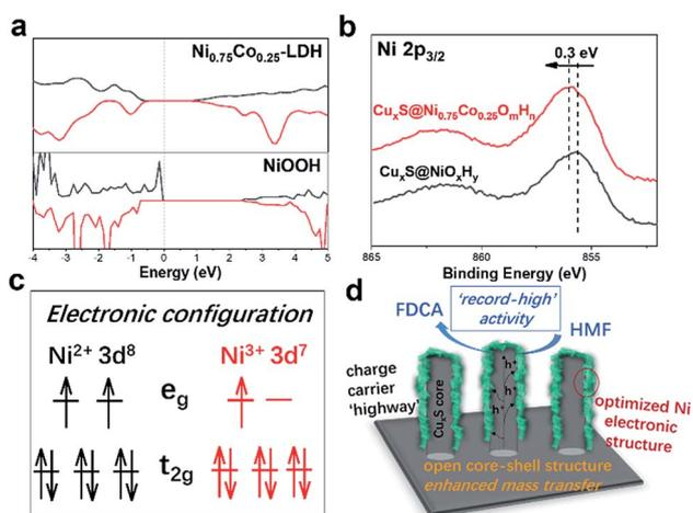
Fig. 4 (a) Projected density of states calculations for  $Ni_{0.75}Co_{0.25}$ -LDH and NiOOH. (b) High resolution Ni 2p<sub>3/2</sub> XPS spectra of  $\text{Cu}_x\text{S}@Ni_{0.75}Co_{0.25}O_mH_n$  and  $\text{Cu}_x\text{S}@NiO_mH_n$ . (c) Schematic illustration of the electronic configuration of the Ni cations with valence states of +2 and +3. (d) Schematic illustration of factors contributing to the high HMF oxidation activity.
