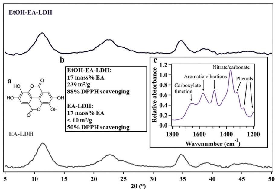
**Fig. 1** The powder X-ray diffraction patterns of EtOH–EA–LDH (upper) and EA–LDH (lower). Insets show (a) the molecular structure of EA, (b) composition, BET specific surface area and DPPH scavenging activity of the LDHs and (c) the snippet of a typical IR spectrum of EA–LDHs indicating the presence of ring-opened EA in the materials. The data are taken from ref. 27.
