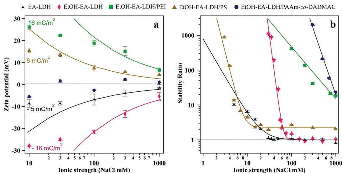
Fig. 4 (a) Zeta potential and (b) stability ratio of the bare and polyelectrolyte-coated LDH particles. Particle concentration was maintained at  $10 \text{ mg L}^{-1}$ . Particles carried polyelectrolyte at doses corresponding to the ASP (shown in Table 1). The solid lines were calculated using eqn (1) in (a) and eqn (2) in (b).
