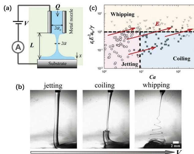
**Fig. 20** (a) Schematic of the experimental setup for an electrified liquid filament in a dielectric liquid with low interfacial tension; (b) representative optical images of “jetting”, “coiling” and “whipping” for the electrified liquid filament under small  $L$ , as the applied field intensity increases, respectively; and (c) a state diagram summarizing the dynamic behaviors of an electrified liquid filament characterized by the capillary and the electrocapillary number.<sup>141</sup>
