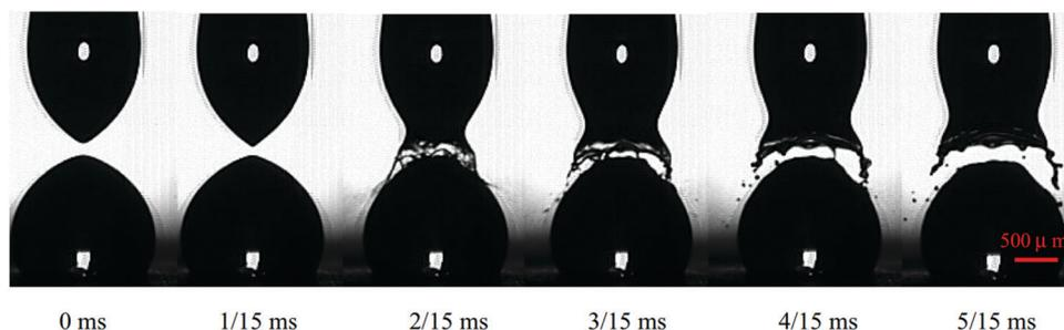
**Fig. 5** Breakup of a water droplet with a conductivity of  $820 \mu\text{S cm}^{-1}$  at a DC voltage of 1.5 kV applied vertically.<sup>113</sup> Reproduced with permission from ref. 113. Copyright 2015, Springer Nature.
