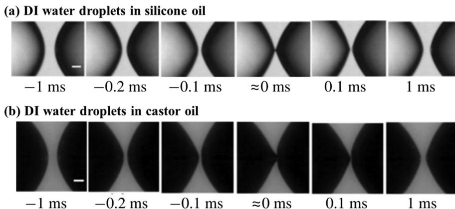
Fig. 6 Non-coalescence of DI water droplets adopting the cone–cone structure in (a) silicone oil and the cone–dimple structure in (b) castor oil under a voltage applied horizontally.<sup>115</sup> Reproduced with permission from ref. 115. Copyright 2018, Cambridge University Press.
