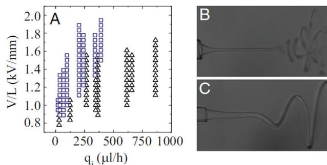
**Fig. 19** (A) State diagram for chaotic and helical whipping of an electrified liquid jet in an immiscible dielectric liquid, characterized by the applied field intensity and the flow rate of the inner liquid (the parameters of the outer phase are kept constant). Representative images of (B) chaotic and (C) helical whipping, in which the outer liquids are silicone oils with a viscosity of 0.5 cP and 9.4 cP, respectively.<sup>218</sup>
