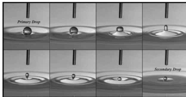
**Fig. 9** The partial coalescence of an aqueous drop and an air/water interface. Each frame is taken 3 ms apart. As the process begins (first frame), the drop shape evolves from a spherical shape to a column (fourth frame) that pinches off and a secondary drop is formed. The time of coalescence begins at the first frame and ends at the seventh frame, where the secondary drop attains a spherical shape. Reproduced with permission from ref. 119. Copyright 2006, AIP Publishing.<sup>119</sup>
