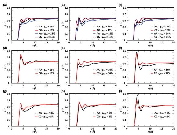
Fig. 3 Comparison of atomistic and CG RDFs of the distances between modified-chitosan and water (W) beads: (a) A-W. (b) B-W. (c) C-W. (d) M-W. (e) MA-W, (f) MB-W, (q) MA-W, (h) MB-W, and (i) MC-W. Note: A, B, and C beads map the GlcN monomers, whereas MA, MB, and MC map the modification groups, as outlined in Section 2.2 and in Fig. 1.
