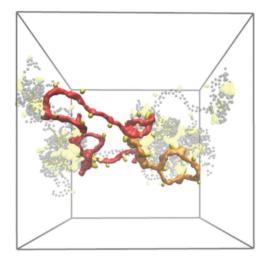
Fig. 10 Simulation snapshot of the cluster-channel morphology in butanoyl-chitosan system with  $\chi_{But}$  = 32%. The butanoyl groups are highlighted in yellow, whereas the polymer backbone is in grey. The conformations of three individual polymer chains are highlighted: one that forms part of a single "cluster" (orange) and two that form bridges between separate clusters (red)
