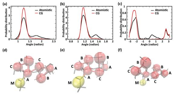
Fig. 5 (a-c) Angle distributions in atomistic and CG models; (d-f) molecular conformations corresponding to the three free energy minima of the  $\varphi - \psi$ dihedral angle conformations in the atomistic model. Atomistic models are drawn as grey sticks, CG beads as red (A, B, and C) and yellow (M) spheres.
