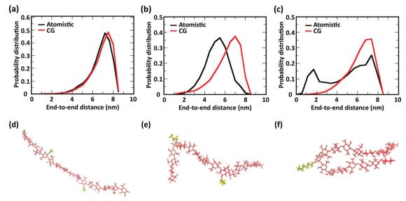
Fig. 6 End-to-end distances sampled in atomistic (black) and CG (red) simulations of single chains of (a) acetyl-chitosan with  $\chi_{Ac} = 16\%$ , (b) butanoylchitosan with  $\chi_{But}$  = 16%, and (c) heptanoyl-chitosan with  $\chi_{Hep}$  = 8%. Simulation snapshots showing compact conformations of single chains (d) acetylchitosan with  $\chi_{Ac} = 16\%$ , (e) butanoyl-chitosan with  $\chi_{But} = 16\%$ , and (f) heptanoyl-chitosan with  $\chi_{Hep} = 8\%$ .
