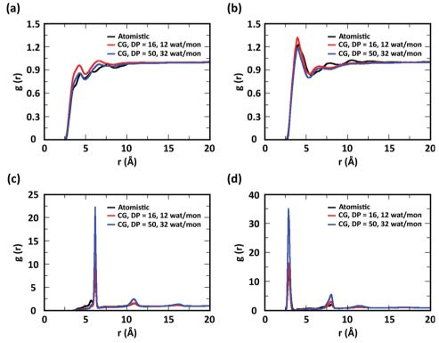
Fig. 7 RDFs for (a) A–WAT, (b) M–WAT, (c) A–A, and (d) A–M bead pairs, obtained from atomistic modeling of acetyl-chitosan with  $\chi_{Ac}$  = 16%, DP = 16, and 12 water molecules per monomer (black), CG modeling of acetyl-chitosan with  $\chi_{Ac}$  = 16%, DP = 16, and 12 water molecules per monomer (red), and CG modeling of acetyl-chitosan with  $\chi_{Ac}$  = 16%, DP = 50, and 32 water molecules per monomer (blue).
