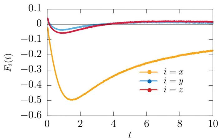
Fig. 13 Time dependence of the  $x$ ,  $y$ , and  $z$  components of the theoretical body force  $\vec{F}(t)$  (eqn (16)) acting on the Janus particle after the temperature quench. Time is given in units of  $t_0 = 10^{-6}$  s.
