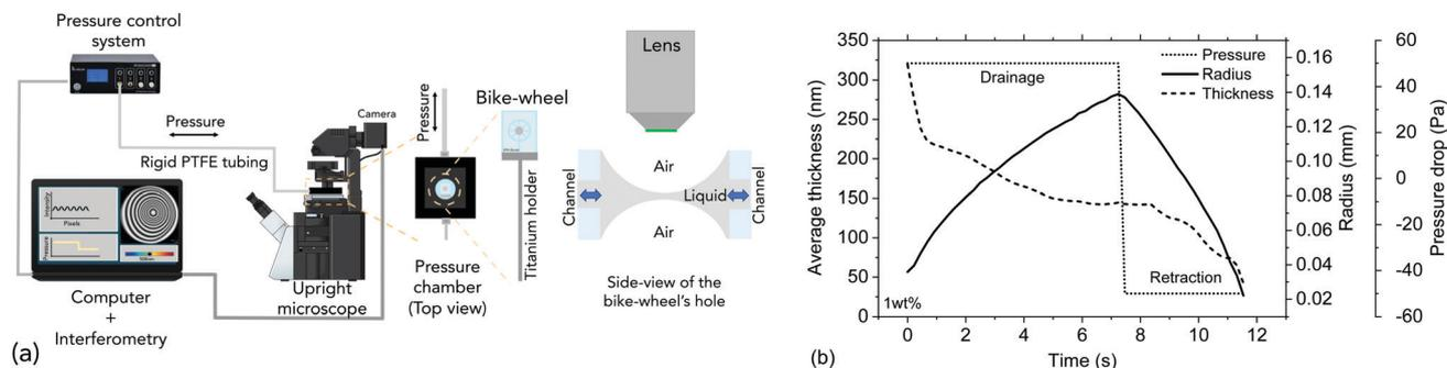
Fig. 2 Experimental approach: (a) the dynamic thin film balance (the various components are explained in the main text). (b) The applied pressure drop  $\pm\Delta P$  and the resulting evolution of film radius and thickness. The time that is allowed for the first phase mimicking drainage is varied during our experiments. The dynamics of the film during “drainage” and “retraction” are monitored by measuring the film dynamics.
