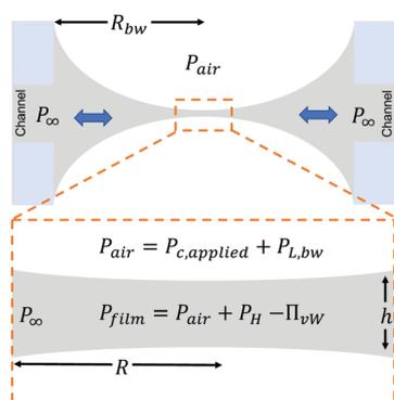
Fig. 3 Pressure contributions in a thin liquid film in the dynamic TFB: the pressure difference  $P_{\text{film}} - P_{\infty}$  drives the inflow and the outflow of liquid.
