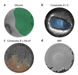
**Fig. 7** Images of the interfaces between a transparent indenter and different samples during pull-off. (a) Silicone,  $E\approx 8.5$  kPa. (b) Composite,  $E\approx 4$  kPa and B=0. (c) Composite,  $E\approx 12$  kPa and  $B\approx 250$  mT. (d) Magneto-rheological fluid,  $B\approx 250$  mT.
