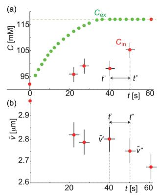
**Fig. 4** Concentration and volume/area measurements on a single GUV. (a) Plot showing  $C_{\rm ex}(t)$  (green) assessed from calcein intensity and  $C_{\rm in}(t)$  (red) assessed from GUV volume during solvent exchange. (b) Plot showing  $\bar{v}(t) = V_{\rm tot}(t)/A_{\rm tot}$  during deflation over time t.
