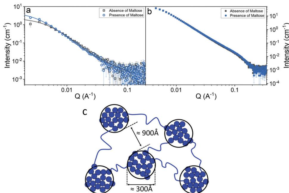
**Fig. 6** SANS curves (a) and SAXS curves (b) of folded MBP hydrogels, (final concentrations: MBP 100 mg ml<sup>-1</sup>, NaPS 30 mM, Ru 100 μm) in the absence (grey) and presence (blue) of 10 mM Maltose. Solid lines show fits to eqn (5). (c) Schematic representation of the predicted structure MBP hydrogels.
