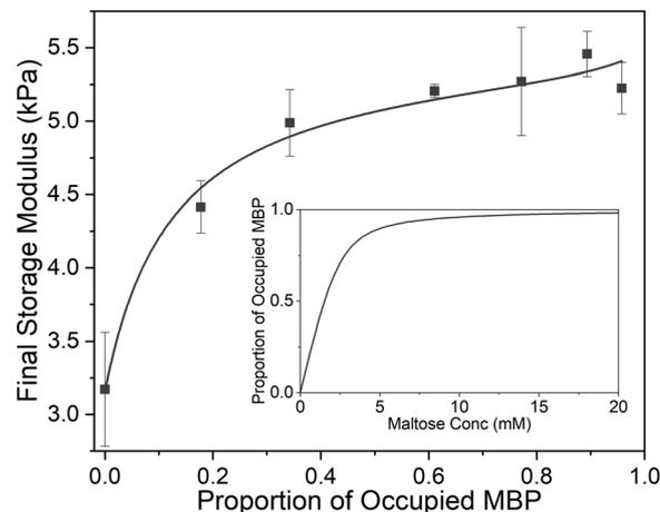
Fig. 5 Final storage modulus as a function of proportion of ligand occupied MBP. Fitted using eqn (1) and (2) (Methods). Where the concentration of MBP,  $\Delta G'$  and  $G_0'$  are taken to be 2.4 mM, 2.25 Pa and 3.16 Pa respectively. (inset) The proportion of occupied MBP as a function of maltose concentration as modelled by eqn (2) using the values 2.4 mM and 800 μM for MBP concentration and apparent MBP: maltose dissociation constant (as extracted from DSC data), respectively.
