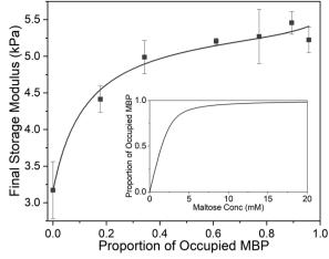
Fig. 5 Final storage modulus as a function of proportion of ligand occupied MBP. Fitted using eqn (1) and (2) (Methods). Where the concentration of MBP,  $\Delta G'$  and  $G_0'$  are taken to be 2.4 mM, 2.25 Pa and 3.16 Pa respectively. (inset) The proportion of occupied MBP as a function of maltose concentration as modelled by eqn (2) using the values 2.4 mM and 800  $\mu$ M for MBP concentration and apparent MBP: maltose dissociation constant (as extracted from DSC data), respectively.
