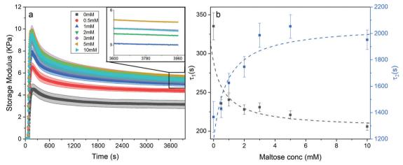
Fig. 7 (a) Gelation curves (showing storage modulus vs. time) of chemical crosslinked MBP hydrogels (final concentrations: 100 mg ml<sup>-1</sup> MBP, 30 mM NaPS,  $100 \mu M$  Ru) as a function of maltose concentration. Illuminated at t = 60 s till t = 360 s. (inset) Magnification of the boxed section in Fig. 7a, with the error bar ribbon removed for clarity. (b) Relaxation time constant of the first and second relaxation mode,  $\tau_1$  (black) and  $\tau_2$  (blue) as a function of maltose
