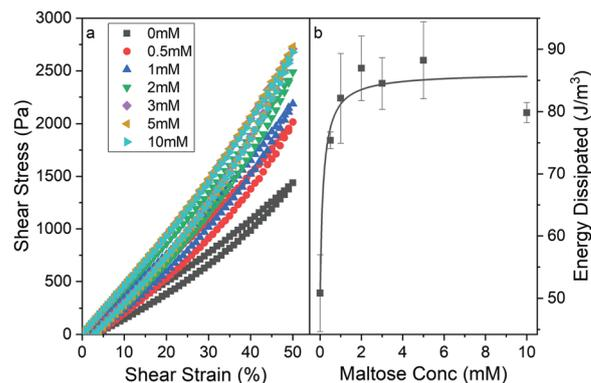
**Fig. 3** (a) Stress–strain curves of chemically crosslinked MBP hydrogels (final concentrations:  $100 \text{ mg ml}^{-1}$  MBP, 30 mM NaPS,  $100 \mu\text{M}$  Ru) as a function of maltose concentration. Samples were strained to 50% at a rate of  $1\%/s$  and then unloaded down to 0% at the same rate. (b) Energy dissipation during load–unload cycle of MBP hydrogels as a function of maltose concentration. Solid line shows fit to Langmuir type model (eqn (S1), ESI<sup>†</sup>).
