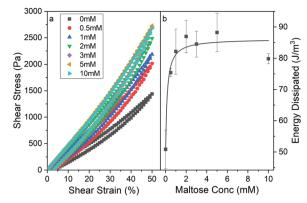
Fig. 3 (a) Stress–strain curves of chemically crosslinked MBP hydrogels (final concentrations: 100 mg ml $^{-1}$  MBP, 30 mM NaPS, 100  $\mu$ M Ru) as a function of maltose concentration. Samples were strained to 50% at a rate of 1%/s and then unloaded down to 0% at the same rate. (b) Energy dissipation during load–unload cycle of MBP hydrogels as a function of maltose concentration. Solid line shows fit to Langmuir type model (eqn (S1), ESI†).
