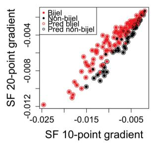
Fig. 5 Results from the best particle channel logistic regression model. Predicted (open circle) and true (filled circle) bijel classification results for each sample in the dataset. Predictions were output from the final particle channel model and plotted as a function of the two variables in the model.
