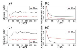
Fig. 2 Comparisons of representative example bijels (in red) and nonbijels (in black) in terms of their structure factors and autocorrelation functions. Panels (a) and (b) show the structure factors and autocorrelation functions of the liquid channel images respectively. Panels (c) and (d) show the structure factors and autocorrelation functions of the particle channel images.
