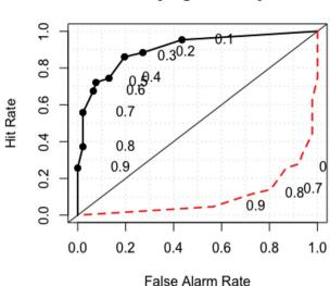
Fig. 7 Receiver operator characteristic curve for the final model fit used to measure the quality of the fitted model. This shows how the true and false negative results change as a function of the probability threshold at which a sample is classed as a non-bijel. The area beneath the curve is 0.912, indicating an excellent model.
