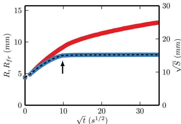
**Fig. 3** Front radius  $R_{fr}$  from a spreading oil drop as determined by tracing the edge of the stain (red circles) and the effective radius  $R$  (blue circles) as determined by the integrated light intensity, both as a function of the square-root of time. On the right axis,  $S^{1/2} (\propto R)$  is given. The integrated intensity contrast  $S$  is proportional to the amount of oil absorbed by the paper. The arrow indicates the point where the total drop is absorbed.
