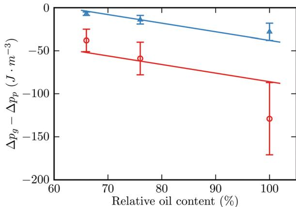
Fig. 9 Difference between oil–grease and oil–paper wetting affinity,  $\Delta p_g - \Delta p_p$ , versus relative oil content of the grease patch for SKF paper (red symbols) and WCP paper (blue symbols). Straight lines are guides to the eye.
