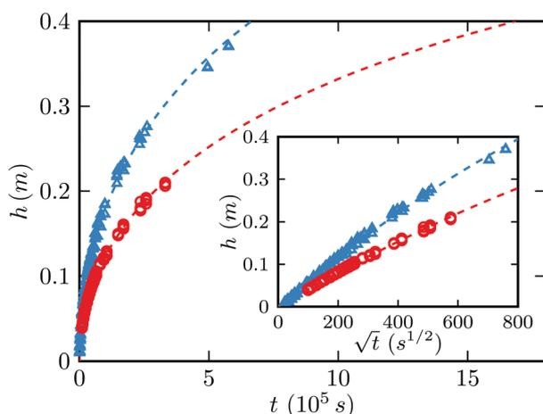
Fig. 6 Rising height of the oil front as a function of time for SKF paper (red symbols) and WCP paper (blue symbols). The insets show the rising height of the oil front *versus* square-root of time. The dashed lines represent the best fits of the capillary rise model.
