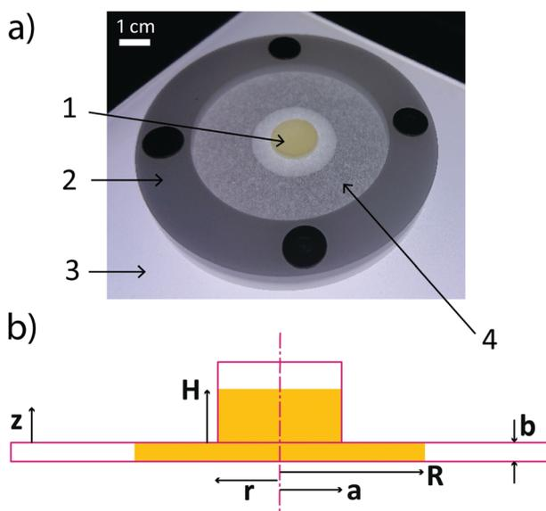
Fig. 1 (a) Experimental setup and (b) its schematic representation (not to scale) of the oil release test. (1) Grease patch with radius  $a$ , (2) paper holder, (3) transmission illumination with a light diffuser, (4) paper with different thickness  $b$ . The bright ring around the grease patch is the growing oil stain with radius  $R$ .
