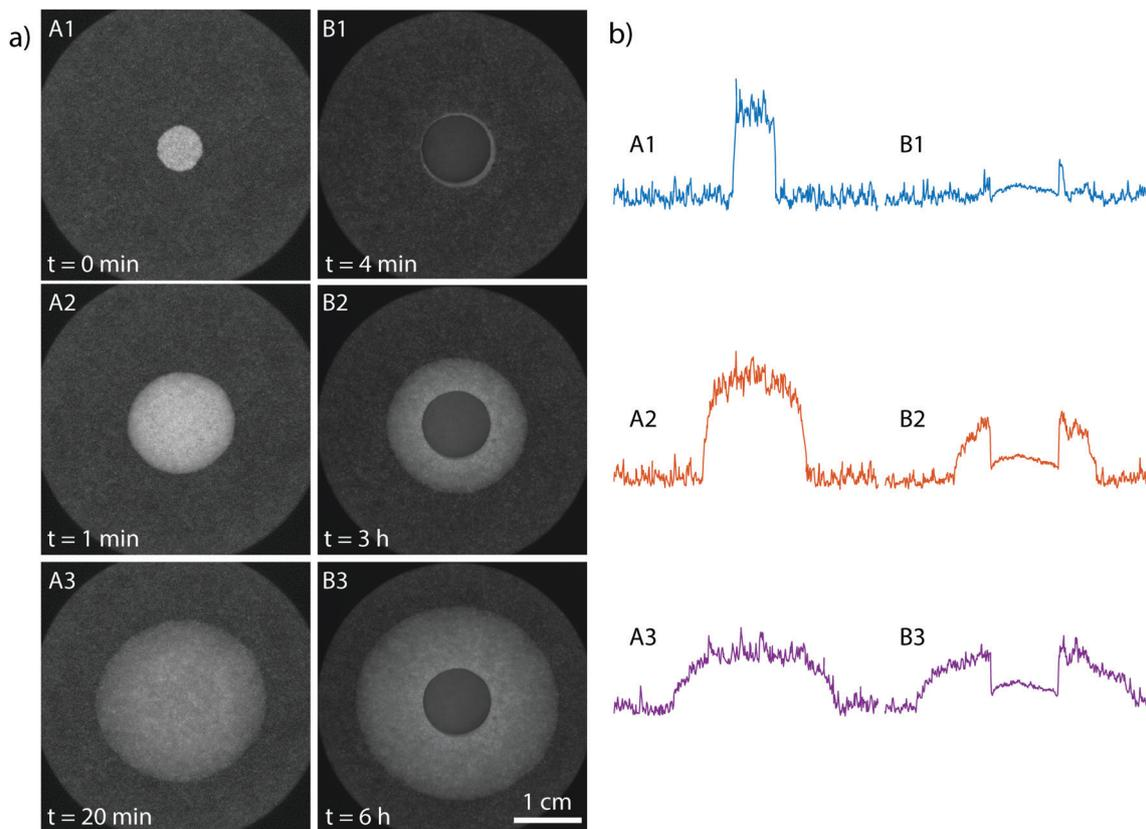
**Fig. 2** (a) Time series of top-view snapshots of the oil stain due to a 10  $\mu\text{L}$  oil drop (A1–A3) and a grease patch containing about 65  $\mu\text{L}$  of oil (B1–B3). (b) The corresponding intensity profiles along a centerline through the stain. Note the dramatic reduction of spreading speed caused by the grease.
