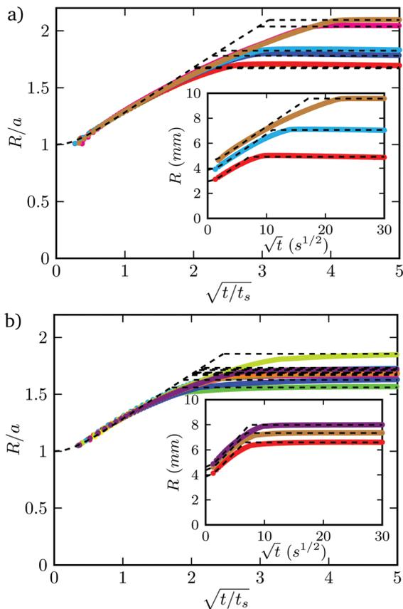
Fig. 7 Normalized effective radius  $R/a$  for the spreading from oil drops of various volumes versus square-root of the normalized time  $\sqrt{t/t_s}$  on SKF paper (panel a) and WCP paper (panel b). Insets: Time dependence of the effective radius  $R$  for oil drops of various volumes. Dashed lines: fits of the oil spreading model.
