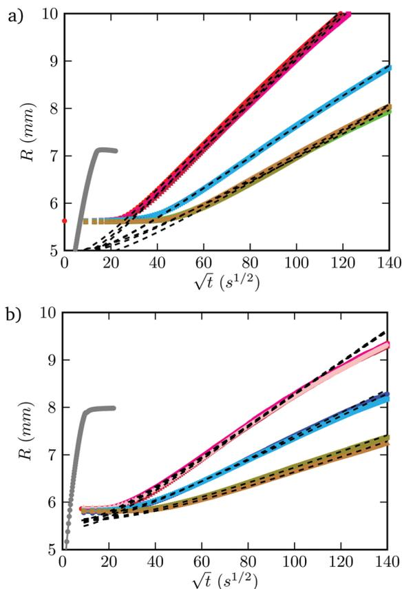
Fig. 5 Effective radius  $R$  versus square-root of time  $\sqrt{t}$  for oil spreading in (a) SKF paper and (b) WCP paper, from a drop (leftmost gray curve) and from grease patches with 100%, 76% and 66% (from upper left to lower right) initial oil content. The colored symbols represent the experimental data. For each concentration, at least three different samples were used, all shown with their own color. The dashed lines represent the best fitting model curves.
