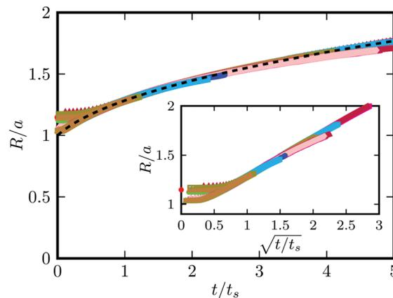
Fig. 8 Normalized radius  $R/a$  of the oil stain as a function of normalized time,  $t/t_s$ , for oil release from a grease patch, showing the collapse of all experimental data, for both SKF paper and WCP paper, to a single master curve. The inset shows  $R/a$  versus  $\sqrt{t/t_s}$ . Color coding corresponds with Fig. 5.
