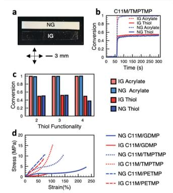
Fig. 2 (a) A comparison of the optical properties of the polydomain LCEs. Nematic genesis (NG) LCE are opaque while isotropic genesis (IG) LCE are transparent. (b) Representative real-time FTIR data monitoring conversion of acrylate and thiol groups in the polymerization of C11M/TMPTMP formulations at temperatures to prepare NG and IG LCE. (c) Summary of overall conversion of acrylate and thiol monomers for each formulation and genesis. (d) Tensile tests of the materials examined here.
