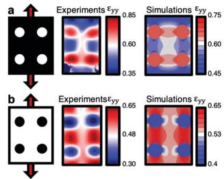
Fig. 7 Local strain measured by DIC and predicted from numerical simulations for (a) IG circles on NG surroundings and (b) NG circles on IG surroundings. At 55% global strain.
