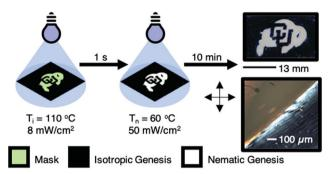
Fig. 4 The approach to prepare patterned regions of IG and NG in polydomain LCE is illustrated. Initially, photopolymerization is localized through a mask for 1-3 seconds in the isotropic state of the mixture. The mask is removed, the sample is cooled into the nematic state, and the material is uniformly exposed to UV light to complete the polymerization reactions. A patterned LCE is illustrated with a buffalo (NG) with the inset "CU" and boundary (IG).
