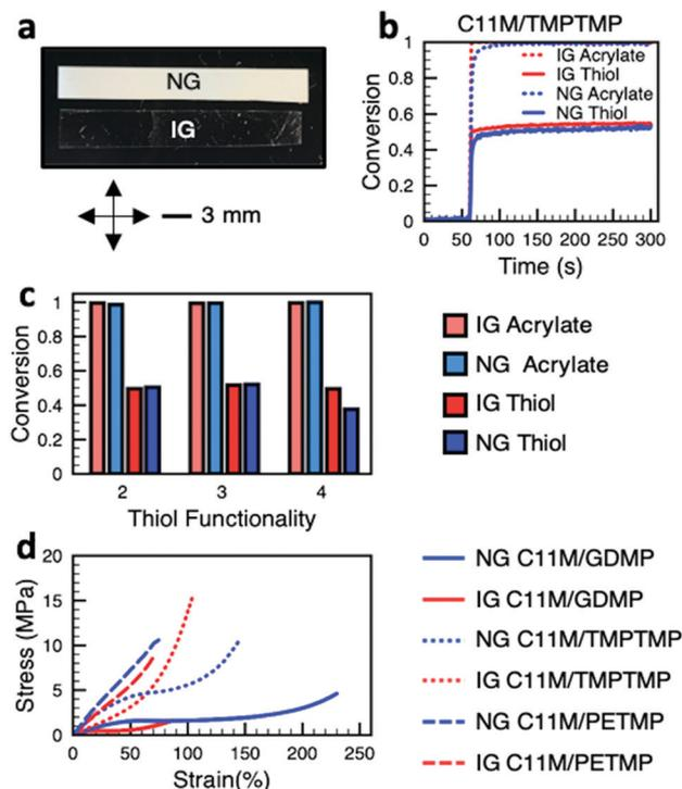
**Fig. 2** (a) A comparison of the optical properties of the polydomain LCEs. Nematic genesis (NG) LCE are opaque while isotropic genesis (IG) LCE are transparent. (b) Representative real-time FTIR data monitoring conversion of acrylate and thiol groups in the polymerization of C11M/TMPTMP formulations at temperatures to prepare NG and IG LCE. (c) Summary of overall conversion of acrylate and thiol monomers for each formulation and genesis. (d) Tensile tests of the materials examined here.
