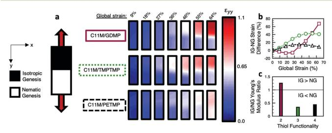
Fig. 5 Digital image correlation (DIC) was used to examine local strain in the materials examined here. (a) Local visualization of strain magnitude (inset legend) in rectangular samples (insert dimensions) as a function of global strain. (b) The difference in strain between the IG and NG regions, taken from the DIC data, is plotted for the three compositions as a function of global strain. (c) The initial ratio of Young's modulus between IG and NG is compared for the three LCE compositions.
