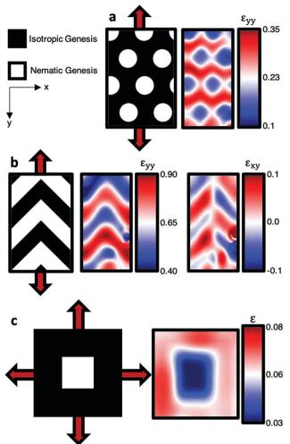
Fig. 6 An LCE prepared from C11M/TMPTMP is patterned with (a) dot patterns, (b) chevron patterns, and (c) a square pattern. Local deformation was characterized with DIC at 27%, 73% global strain, and 5% global strain, respectively
