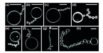
Fig. 4 Multispherical shapes consisting of one large sphere and a linear or branched chain with  $N_s \ge 4$  small spheres: (a-c) linear chains with (a)  $N_s = 4$ , (b)  $N_s = 5$ , and (c)  $N_s = 6$ . (d-h) Branched chains with (d)  $N_s = 7$ , (e and f)  $N_s = 8$ , (g)  $N_s = 14$  and (h)  $N_s = 15$ . Various sugar concentrations; all scale bars are 10 µm.
