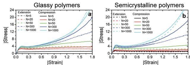
Fig. 2 The magnitude of true stress in units of  $\epsilon_{LJ}/\sigma^3$  versus true strain magnitude from uniaxial compression (solid lines) and tensile (dashed lines) deformation of (a) glassy and (b) semicrystalline polymers with chain lengths  $N = 5, 20, 50, 300$  and  $1000$  as given in the legends.
