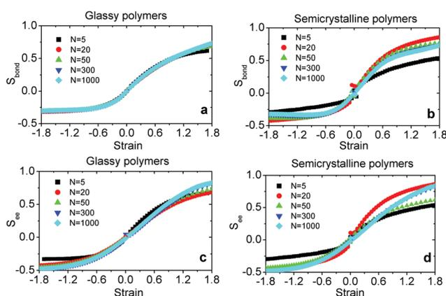
Fig. 5 The global nematic order parameter of bonds  $S_{\text{bond}}$  for glassy (a) and semicrystalline (b) polymers of different chain lengths,  $N$ , as a function of strain in both compression (negative strain) and tensile deformation modes. Likewise, the strain-dependence of the nematic order parameter of chains end-to-end vector  $S_{\text{ee}}$  for glassy (c) and semicrystalline (d) polymers.
