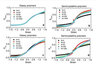
Fig. 5 The global nematic order parameter of bonds  $S_{bond}$  for glassy (a) and semicrystalline (b) polymers of different chain lengths, N, as a function of strain in both compression (negative strain) and tensile deformation modes. Likewise, the strain-dependence of the nematic order parameter of chains end-to-end vector See for glassy (c) and semicrystalline (d) polymers.
