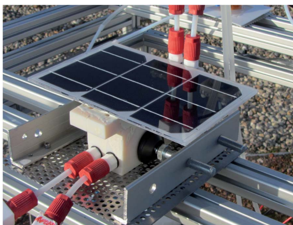
Fig. 1 Close-up of a device similar to the analysed one (except for the different plastic used in the electrolyser casing) in the measurement setup. Electrolyte inlets at the bottom of the electrolyser, outlets at the top.
