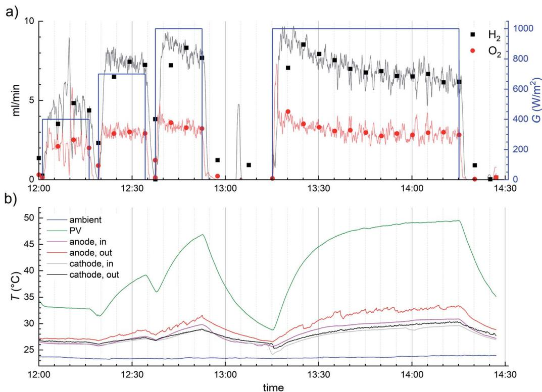
Fig. 6 Time dependent profiles measured indoors of (a) H<sub>2</sub> and O<sub>2</sub> flow rates and solar irradiance transients. Flow rate transients are averaged over 60 seconds (lines) and 5 minutes (squares and circles) to reduce noise in the signal. (b) Time dependent profiles of ambient, PV and electrolyte temperatures.
