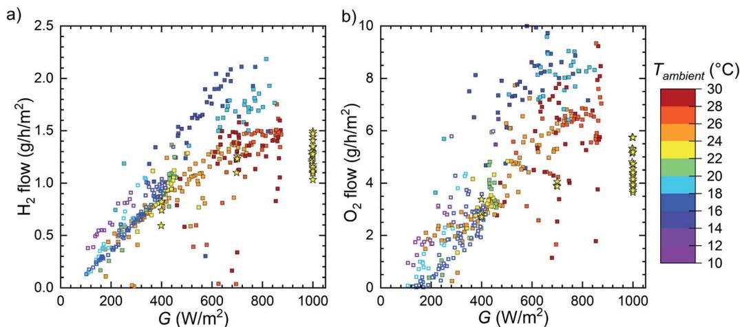
Fig. 11 (a) The hydrogen flow rate and (b) oxygen flow rate as a function of irradiance, assuming that the outflows are pure  $H_2$  and  $O_2$ . Pure  $H_2$  and  $O_2$  outflows at 2.0  $H_2 : O_2$  molar ratio would correspond to 4.0 g of  $O_2$  per 1.0 g of  $H_2$ . Outdoor data marked with squares (open squares 22 to 24.10.2019), indoor with stars.
