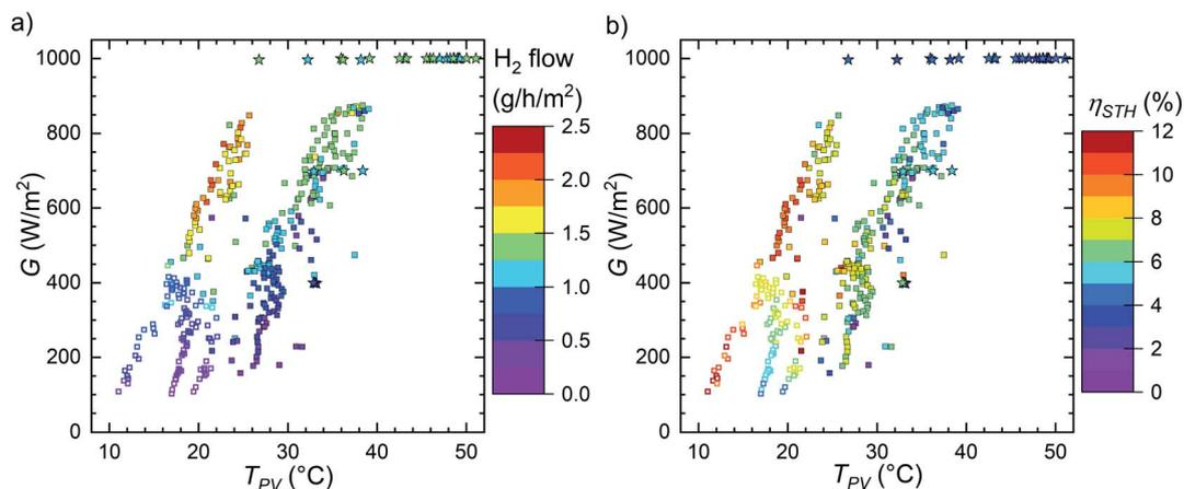
Fig. 8 (a) The  $H_2$  generation rate and (b) the STH efficiencies as the function of the measured temperature of the PV and the irradiance. The values are a consolidation of indoor and several outdoor measurement campaigns on various days with a variety of weather conditions. Outdoor data (front glass) marked with squares, indoor data (back of the PV) with stars, open squares indicate the measurement on 22 to 24.10.2019 (Fig. S4.6–S4.8†).
