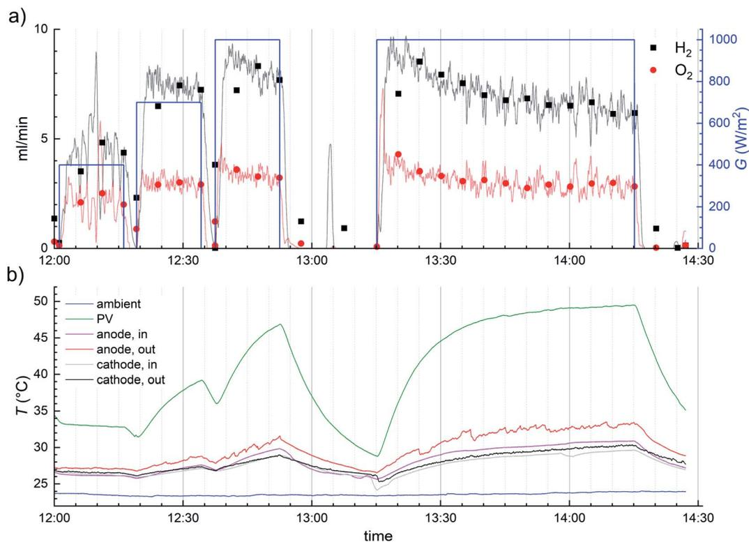
Fig. 6 Time dependent profiles measured indoors of (a)  $\text{H}_2$  and  $\text{O}_2$  flow rates and solar irradiance transients. Flow rate transients are averaged over 60 seconds (lines) and 5 minutes (squares and circles) to reduce noise in the signal. (b) Time dependent profiles of ambient, PV and electrolyte temperatures.
