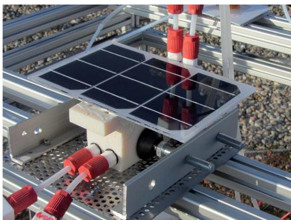
Fig. 1 Close-up of a device similar to the analysed one (except for the different plastic used in the electrolyser casing) in the measurement setup. Electrolyte inlets at the bottom of the electrolyser, outlets at the top.
