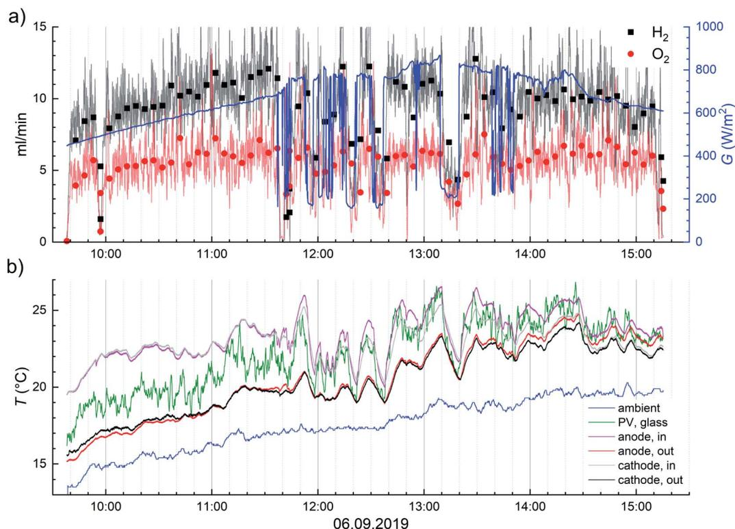
Fig. 5 Time dependent profiles measured on 6<sup>th</sup> September 2019 in Berlin, Germany of (a)  $\text{H}_2$  and  $\text{O}_2$  flow rates and solar irradiance transients. Flow rate transients are averaged over 60 seconds (lines) and 5 minutes (squares and circles) to reduce noise in the signal. (b) Time dependent profiles measured on 6<sup>th</sup> September 2019 of ambient, PV glass and electrolyte temperatures.
