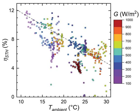
Fig. 9 The solar to hydrogen conversion efficiency,  $\eta_{STH}$  as a function of the ambient temperature, divided into groups of different irradiances. Outdoor data marked with squares (open squares 22 to 24.10.2019), indoor data with stars. The dashed line indicates a  $-0.35\% \text{ } ^\circ\text{C}^{-1}$  slope.
