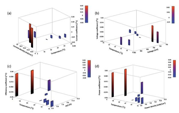
Fig. 9 3D bar plot of the (a) current coefficient, (b) voltage coefficient, (c) efficiency coefficient, and (d) power coefficient at the specific temperature and corresponding parameters for  $S_T$  devices.
