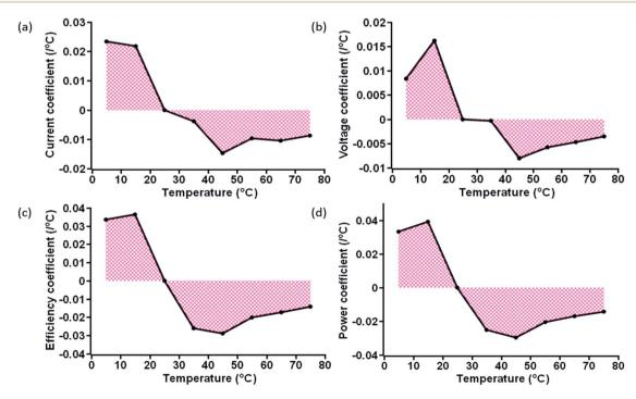
Fig. 7 Area plot of the variation of the (a) current coefficient, (b) voltage coefficient, (c) efficiency coefficient, and (d) power coefficient at specific temperatures for  $S_T$  devices.
