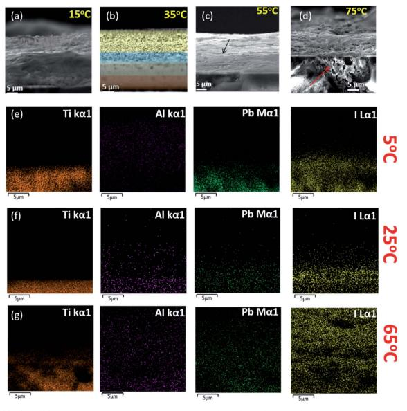
Fig. 4 (a), (b), (c), and (d) are the SEM images of  $S_T$  testing devices at 15 °C, 35 °C, 55 °C, and 75 °C, respectively. (e), (f), and (g) are energy dispersive X-ray (EDX) elemental colour maps of Ti, Al, Pb, and I of the devices at 5 °C, 25 °C, and 65 °C, respectively.
