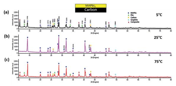
Fig. 11 (a), (b), and (c) XRD data of glass samples coated with WO<sub>3</sub> doped carbon and perovskite at 5 °C, 25 °C, and 75 °C, respectively showing the formation of an intermediate state
