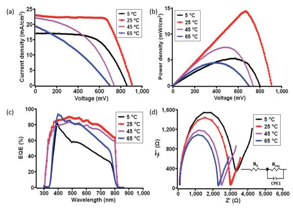
Fig. 6 (a) Current density-voltage curves and (b) power density-voltage curve for the best  $T_T$  c-PSC at different temperatures in the range of 5 to 75 °C. Photovoltaic characterization of the best T<sub>T</sub> device for each temperature in the range of 5 °C to 75 °C, (c) IPCE spectra of c-PSCs at different temperatures, and (d) corresponding EIS characteristics (Nyguist plots) with the fitted circuit diagram for the  $T_T$  device having the best performance.
