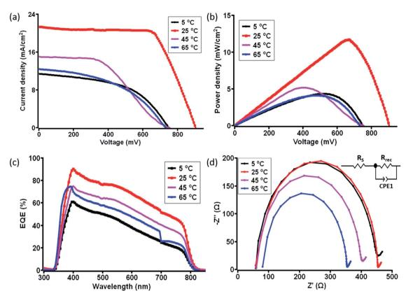
Fig. 5 (a) Current density-voltage (J-V) curves and (b) power density-voltage curve for the  $S_T$  c-PSCs at different temperatures in the range of 5 °C to 75 °C, (c) IPCE spectra of c-PSCs at different temperatures, and (d) corresponding EIS characteristics (Nyquist plots) with the fitted circuit diagram for  $S_T$  devices having the best performance.
