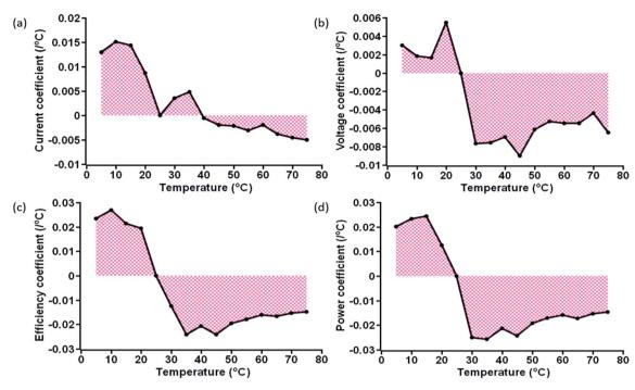
Fig. 8 Area plot of the variation of the (a) current coefficient, (b) voltage coefficient, (c) efficiency coefficient, and (d) power coefficient at specific temperatures for  $T_{\top}$  devices.
