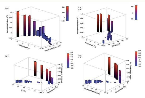
Fig. 10 3D bar plot of the (a) current coefficient, (b) voltage coefficient, (c) efficiency coefficient, and (d) power coefficient with respect to temperature, and corresponding parameters for  $T_T$  devices.
