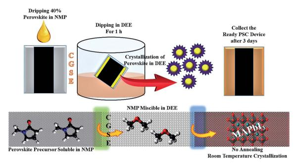
Fig. 1 Schematic illustration showing the CGSE process for the room-temperature deposition of the MAPbl<sub>3</sub> thin film to fabricate the c-PSC. The process of perovskite formation without any heat treatment was performed for three days for fine crystallization. Exchange of N-methyl-2pyrrolidone (NMP) with diethyl ether (DEE) helped in the formation of the pure crystal phase (the yellow arrows represent the crystal growth process by changing the solvent medium).
