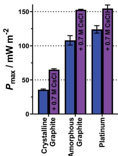
Fig. 9 Bar chart showing the  $P_{\text{max}}$  for 0.2 M  $\text{K}_3[\text{Fe}(\text{CN})_6]$  and 0.2 M  $\text{K}_4[\text{Fe}(\text{CN})_6]$  equimolar thermocell, using three different electrode materials; crystalline graphite, amorphous graphite and platinum, without (blue bars) and with (purple bars) 0.7 M CsCl present in the electrolyte. All measured at an applied  $\Delta T = 18 \text{ K}$  ( $T_{\text{cold}} = 17 \text{ }^\circ\text{C}$ ).
