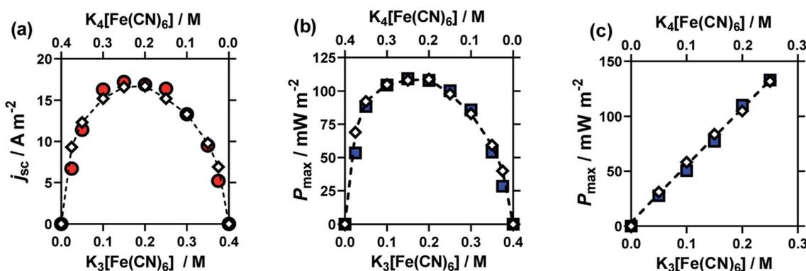
Fig. 5 Plots overlaying the experimental data points (coloured circles and squares) with Butler-Volmer modelled data points (white diamonds), for the non-equimolar ratio study, for (a) the  $j_{\text{sc}}$  and (b)  $P_{\text{max}}$ . Also shown in (c) are the experimental and modelled  $P_{\text{max}}$  data for the equimolar concentration study. All modelled data used  $k_{\text{agg}} = 1.68 \times 10^{-4} \text{ cm s}^{-1}$ , with all other parameters matching experimental conditions.
