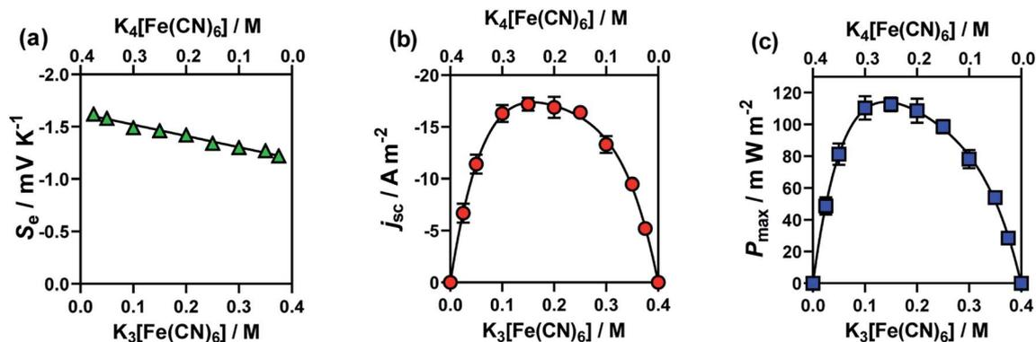
Fig. 3 Plots (a)–(c) showing the effect of changing the ratio of  $[\text{Fe}(\text{CN})_6]^{3-}$  to  $[\text{Fe}(\text{CN})_6]^{4-}$  upon (a) the  $S_e$  coefficient (green triangles); (b) the  $j_{sc}$  (orange circles) and (c) the  $P_{max}$  (blue squares). The concentrations of the redox couples were varied whilst maintaining a summed concentration of 0.4 M, where error bars represent 1 SD (not shown if bars smaller than symbol). All other experimental conditions as per Fig. 1.
