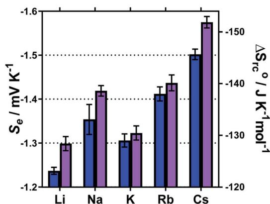
Fig. 7 Bar chart showing the measured  $S_e$  and calculated corresponding redox-couple entropy changes ( $\Delta S_{rc}$ ) for 5 mM of  $\text{K}_3[\text{Fe}(\text{CN})_6]$  and 5 mM  $\text{K}_4[\text{Fe}(\text{CN})_6]$  in the presence of either 0.4 M  $\text{X}_2\text{SO}_4$  (blue) or 1 M  $\text{XCl}$  (purple) where  $\text{X}$  is shown as either  $\text{Li}$ ,  $\text{Na}$ ,  $\text{K}$ ,  $\text{Rb}$  or  $\text{Cs}$ . All values determined using a non-isothermal platinum thermocell.
