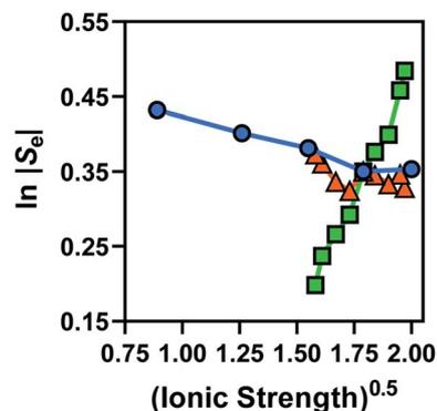
Fig. 4 Plots of the measured  $\ln|S_e|$  vs. the (ionic strength)<sup>0.5</sup> of that particular solution, for the concentration study of equimolar  $[\text{Fe}(\text{CN})_6]^{3-/4-}$  (blue circles), non-equimolar concentrations of  $[\text{Fe}(\text{CN})_6]^{3-}$  to  $[\text{Fe}(\text{CN})_6]^{4-}$  (green squares) and the ‘Nernstian corrected’ form of the non-equimolar data to yield ‘ $S_e^*$ ’ (red triangles).
