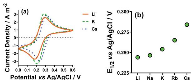
Fig. 6 Showing (a) Cyclic voltammograms (CVs) recorded for 5 mM  $\text{K}_3[\text{Fe}(\text{CN})_6]$  and 5 mM  $\text{K}_4[\text{Fe}(\text{CN})_6]$  in the presence of 0.4 M  $\text{M}_2\text{SO}_4$  ( $\text{M} = \text{Li}^+$  (orange solid line),  $\text{K}^+$  (green dashed line) and  $\text{Cs}^+$  (blue dotted line)) and (b) the trend in  $E_{1/2}$  extracted from the CVs for all five alkali metal cations. All recorded at a Pt electrode at  $50 \text{ mV s}^{-1}$  and room temperature.
