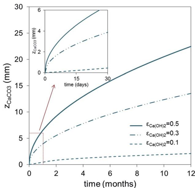
Fig. 3 Evolution with time of the carbonated layer ( $z_{\text{CaCO}_3}$ ) in carbonated solids according to eqn (2), for different porosities ( $\epsilon_{\text{Ca(OH)}_2}$ ) and assuming a  $\text{CO}_2$  concentration gradient of 400 ppmv at 20 °C.
