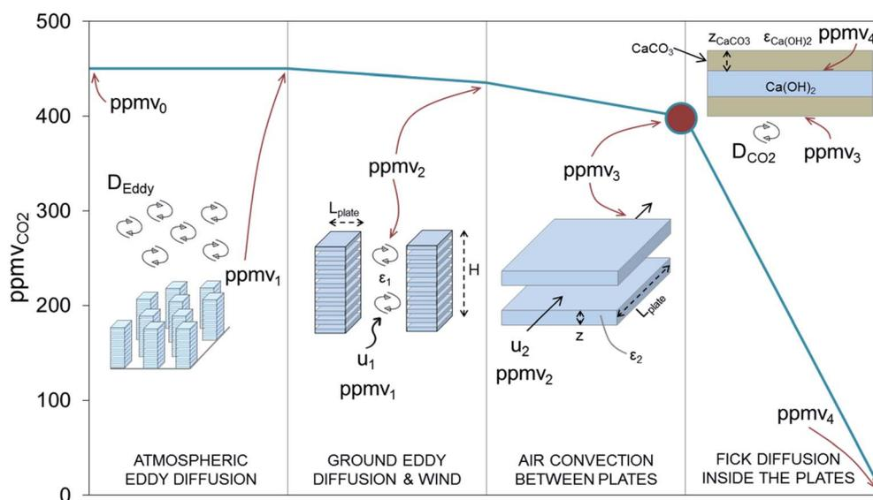
Fig. 4 Evolution of the  $\text{CO}_2$  concentration in air through the different  $\text{CO}_2$  transport/diffusion stages, taking place at increasing scales from right to left: interior of a plate, individual plates, stacked plates and numerous stacked plates arranged in a field.
