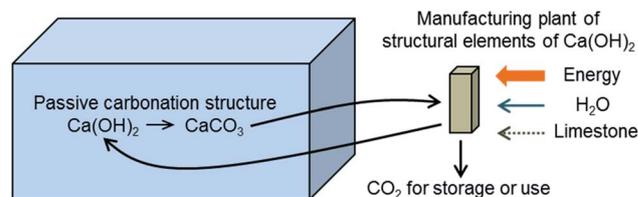
Fig. 2 The concept of passive  $\text{CO}_2$  capture from air by the carbonation of a suitable structure of solid  $\text{Ca}(\text{OH})_2$  exposed to ambient air.
