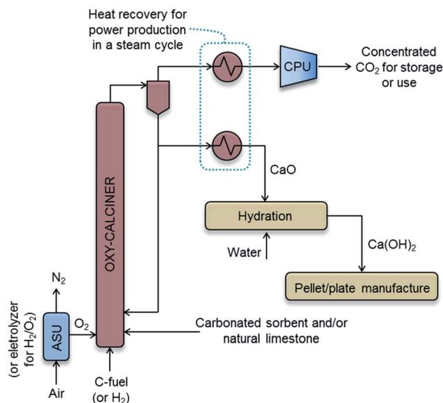
Fig. 5 General process scheme of the oxy-fired CFB calcination system and Ca(OH)<sub>2</sub> manufacture.
