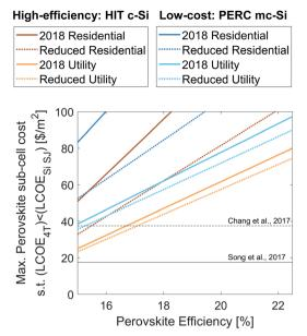
Fig. 4 Maximum added areal cost of adding the perovskite top cell to the bottom Si SJi bottom cell and the high-efficiency HIT c-Si cell in the cases of current and reduced system costs for residential and utility
