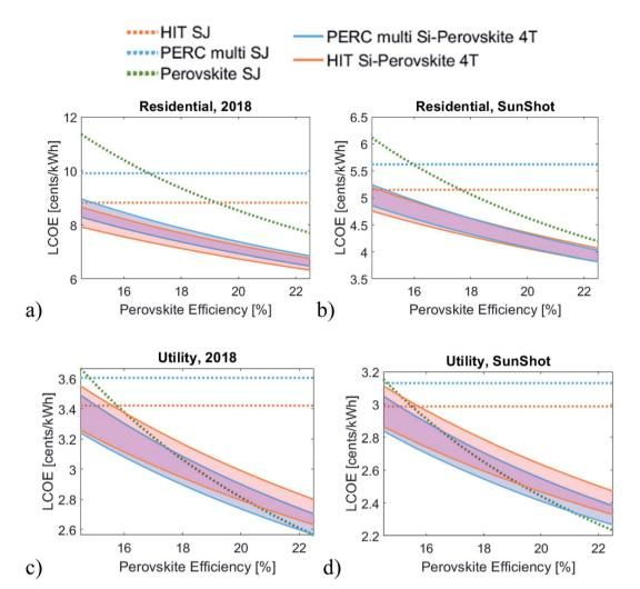
Fig. 3 LCOE of each single-junction and 4T tandem architecture versus perovskite assuming (a) 2018 residential cost, (b) reduced residential BOS cost scenario, (c) 2018 utility costs, (d) reduced utility BOS cost scenario. The two tandem LCOE values are calculated using a range of subbandgap transmission, 70.5-90%.
