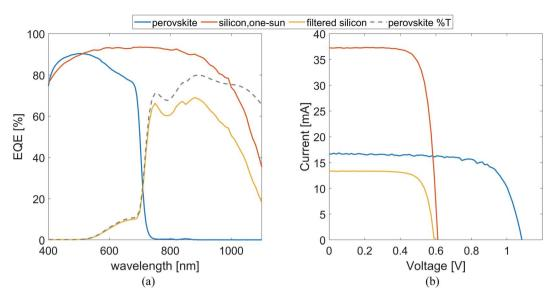
Fig. 2 (a) External quantum efficiency (EQE) and (b) current–voltage (JV) curve of the perovskite top cell, the silicon bottom cell under one-sun illumination, and the silicon bottom cell under one-sun filtered by the perovskite top cell.
