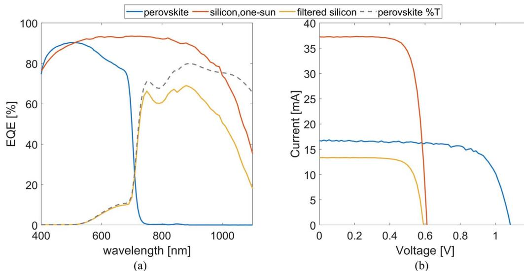
Fig. 2 (a) External quantum efficiency (EQE) and (b) current–voltage ( $JV$ ) curve of the perovskite top cell, the silicon bottom cell under one-sun illumination, and the silicon bottom cell under one-sun filtered by the perovskite top cell.
