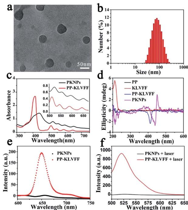
**Fig. 1** Self-assembly of PP-KLVFF into PKNPs. (a) TEM image of PKNPs. (b) DLS histogram of PKNPs. (c) UV-vis absorption spectra of PP-KLVFF and PKNPs. The inset shows the amplified absorption spectra of Q bands. (d) CD spectra of PP, KLVFF, PP-KLVFF, and PKNPs. (e) Fluorescence emission spectra ( $\lambda_{\text{ex}}$ : 450 nm) of PKNPs and PP-KLVFF. (f) ROS generation by PKNPs and PP-KLVFF, using DCFH-DA (10  $\mu$ M) as a probe ( $\lambda_{\text{ex}}$ : 488 nm).
