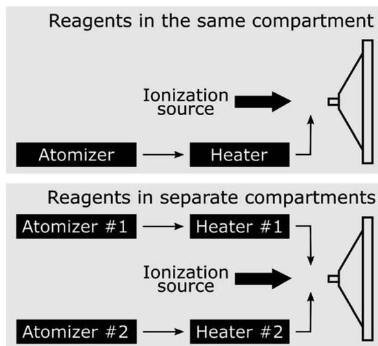
Fig. 7 (a) 'Reagents in the same compartment' and (b) 'reagents in separate compartments' setups, as designed by Jacobs *et al.*<sup>87</sup>
