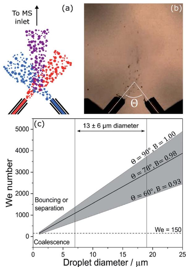
Fig. 6 Schematics (a) and still frame (b) from Lee *et al.*<sup>46</sup> showing the microdroplet fusion mass spectrometry setup. (c) Weber number ( $We$ ) calculated for the collision of two equally-sized aerosol droplets with variable colliding angle,  $\theta$ ; the diameter range of  $13 \pm 6 \mu\text{m}$  indicated by Lee *et al.*<sup>46</sup> is shown for reference. The horizontal dashed line at  $We = 150$  separates regions where coalescence or bouncing/separation are expected to occur.
